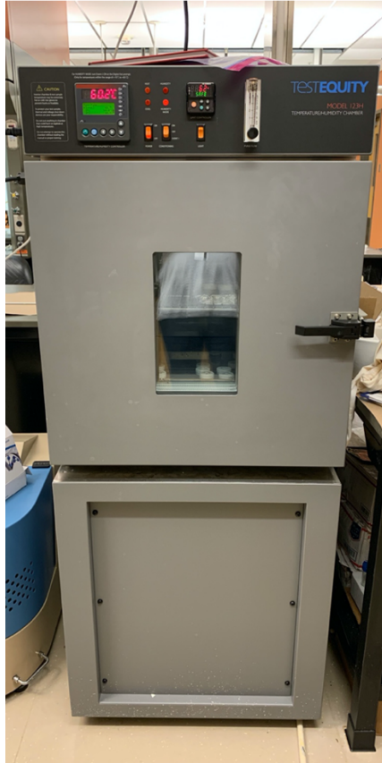
Figure 3.10 TestEquity Controlled Temperature and Humidity Chamber (TestEquity 123H Controlled Temperature and Humidity Chamber, TestEquity, CA) for curing geopolymer composite samples.
