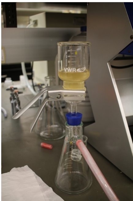
Figure 3.23 Vacuum filtration setup used to measure the TDS in the laboratory and determine the conductivity factor.
