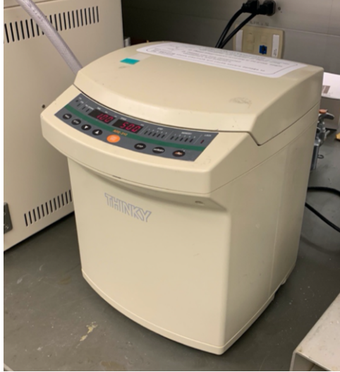
Figure 3.7 Thinky Mixer (ARE-310, Thinky, CA) used for mixing geopolymer slurry.
