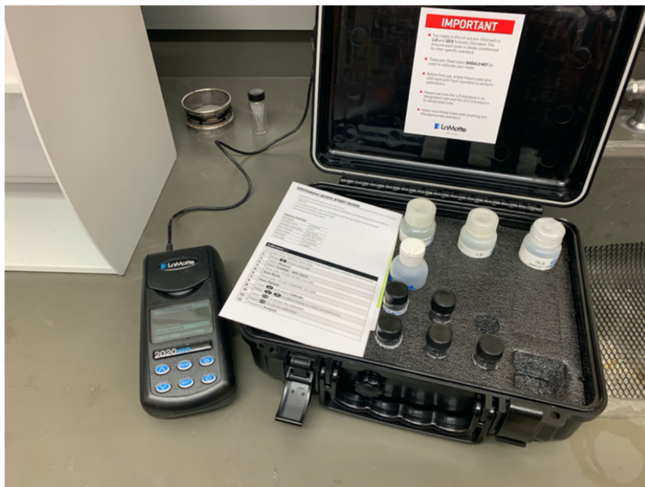
Figure 3.22 LaMotte 1970-EPA Model 2020we Portable Turbidity Meter (LaMotte Company, Chestertown, MD) used to measure turbidity in this study.
