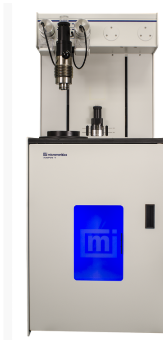
Figure 3.20 Autopore V, Mercury Intrusion Porosimeter (Micromeritics, Norcross, GA) used for porosity analysis in this study.
