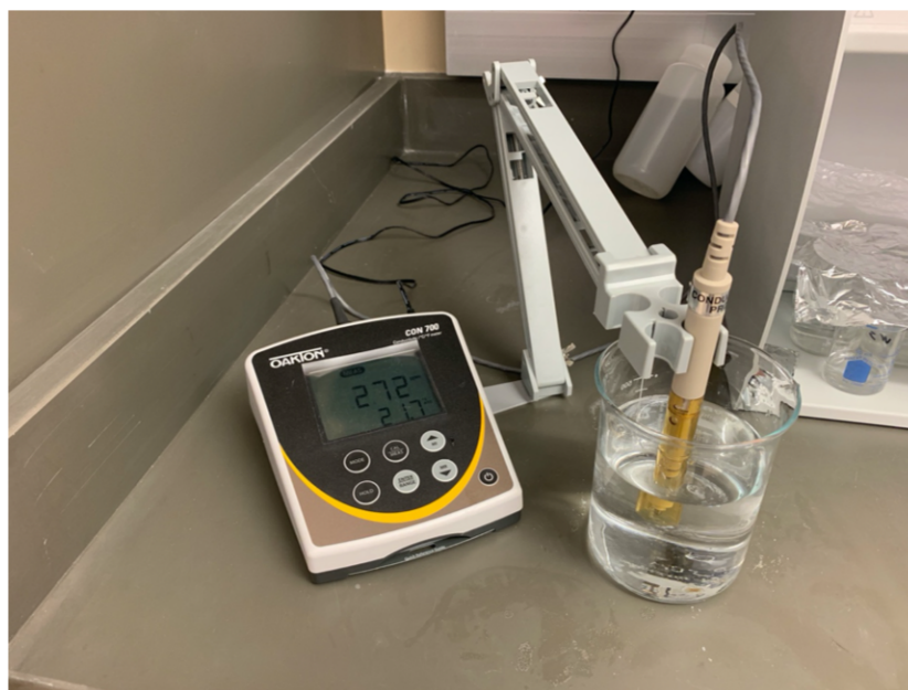
Figure 3.24 Conductivity meter (Oakton Con 700 Total Dissolved Solid meter, Oakton Instruments, Vernon Hills, IL) used in this study.
