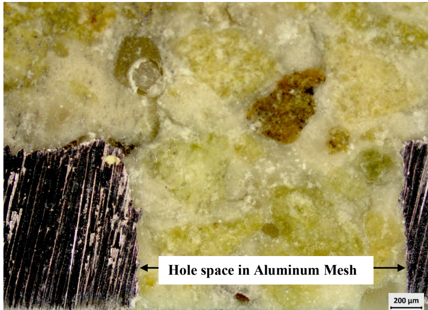
Figure 4.4 Optical micrograph of the cross-section of a geopolymer composite membrane showing the presence of geopolymer matrix and zeolite particles in the holes of the aluminum mesh support.
