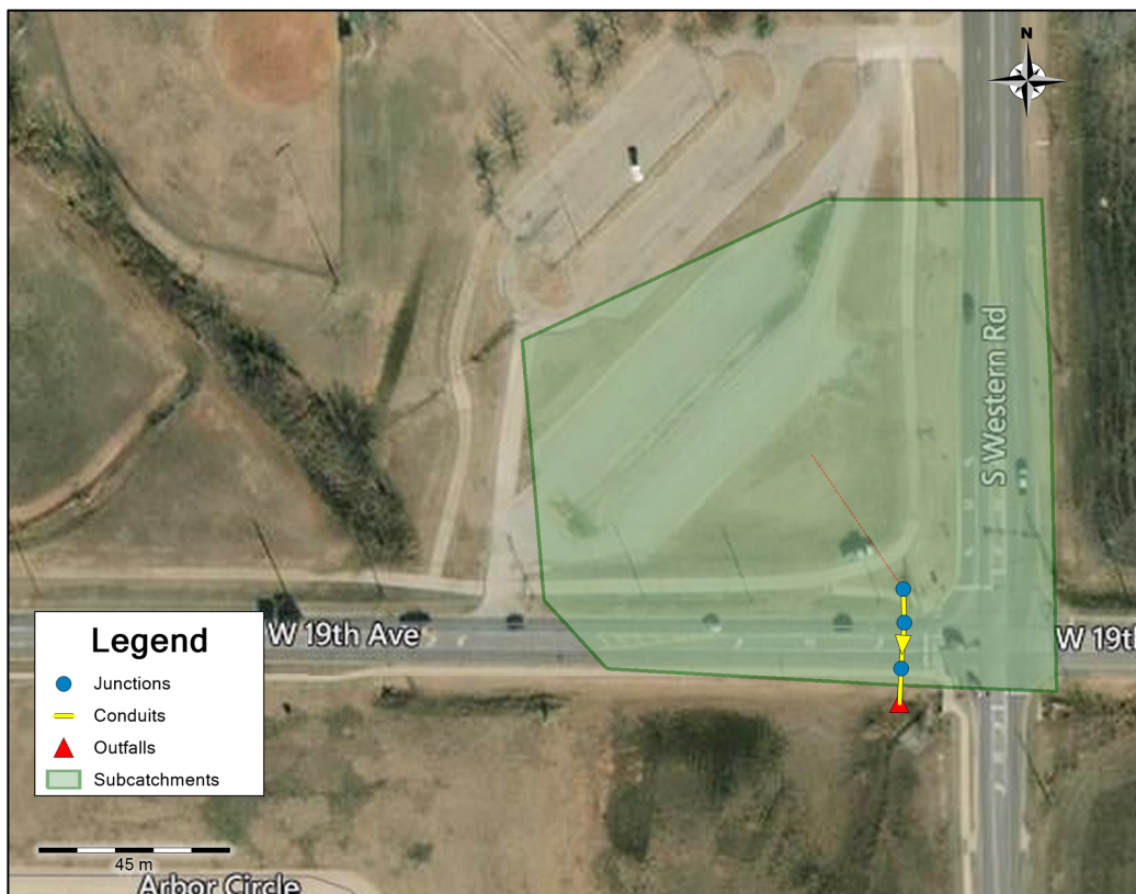
Figure 11. A map of the PCSWMM simulation study area at Babcock Park in Stillwater, Oklahoma. The subcatchment, junctions, conduits, and outfall are shown in the photo (CHI, 2021).
