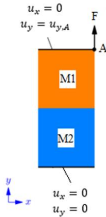
Figure 2.8 Boundary conditions of the FEA model
