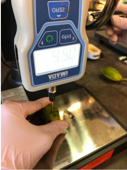
Figure 3.3. Measuring pecan shell firmness using force gauge with a 2mm probe needle.
