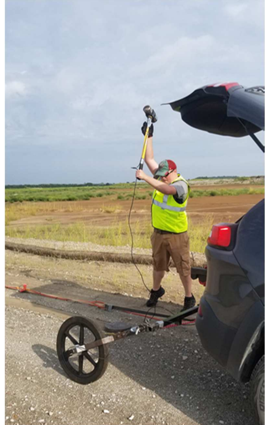
Figure 7. Field photos of electrical resistivity data acquisition (left) and seismic data acquisition (right).
