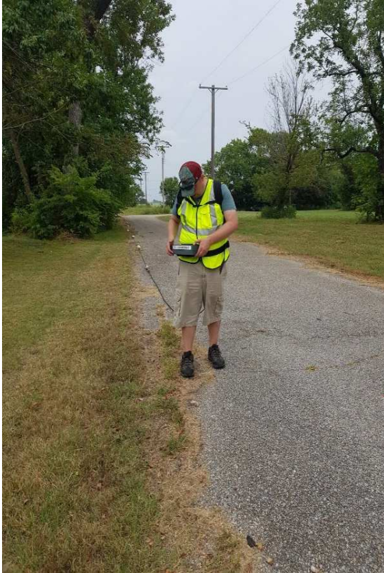
Figure 7. Field photos of electrical resistivity data acquisition (left) and seismic data acquisition (right).
