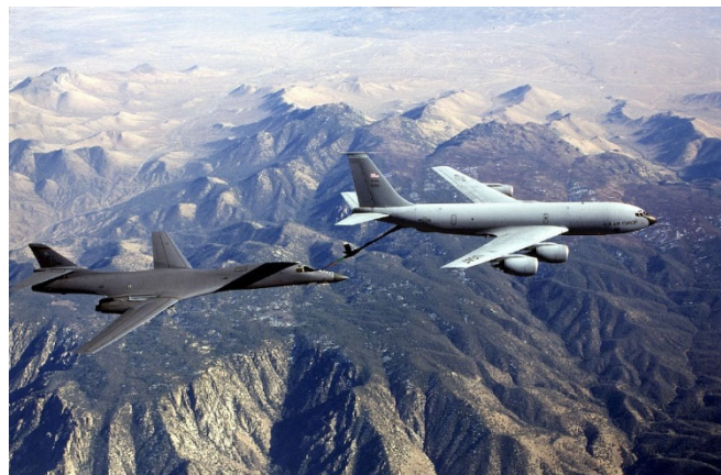
Figure 2. KC-135 utilizing boom refueling to perform AAR on a B-1 Lancer
