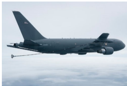
Figure 1. KC-46 utilizing hose-and-drogue refueling to perform AAR
