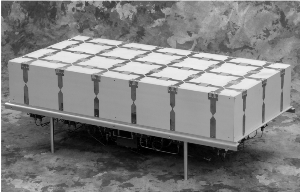
Figure 2.14: Interdigitally-coupled dipole array making use of tight-coupling. Taken from [28].
