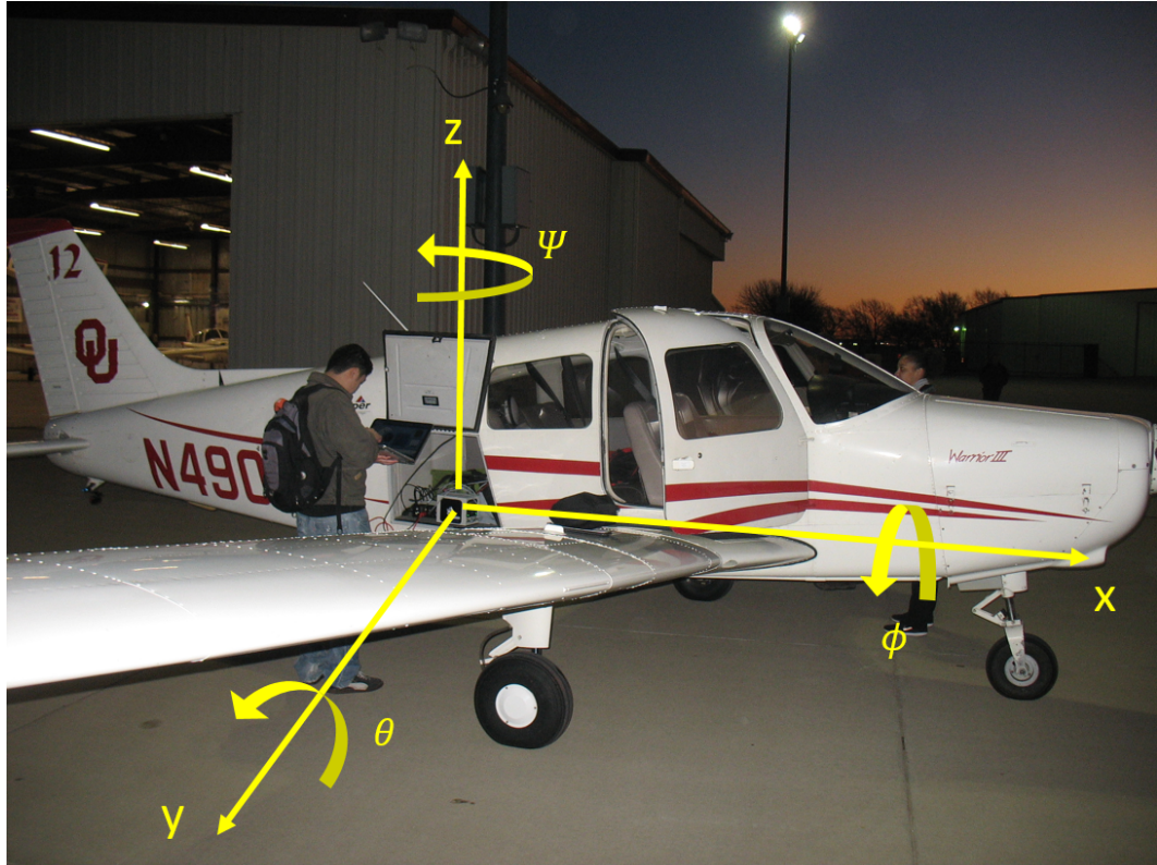
Figure 2.4: Euler angles defined as rotations around the axis as follows: Roll ( \phi ) is the rotation around X , Pitch ( \theta ) is the rotation around Y , and Yaw ( \psi ) is the rotation around Z .
