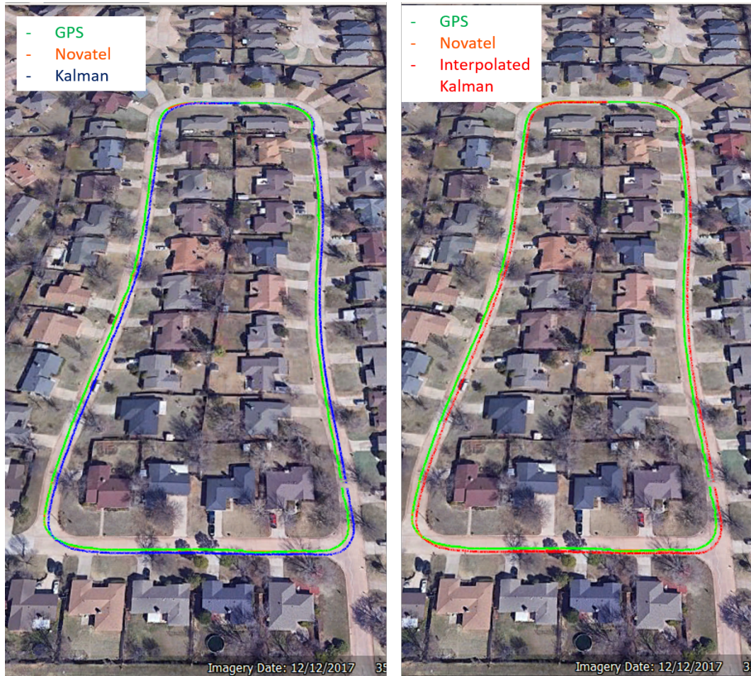
Figure 5.19: Kalman algorithm results. The left image shows the Kalman results plotted on top of the GPS coordinates and the navigation solution given by the NovAtel system. The right image shows the Kalman interpolated results plotted on top of GPS and NovAtel coordinates. These maps are obtained using Google Earth.
