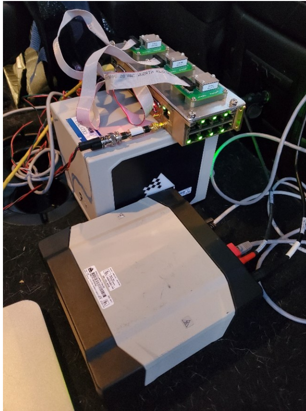
Figure 5.22: An image of the multi-IMU instrumentation setup. The gold box mounted on the NovAtel IMU is the ARENA CTU and the silver boxes with the ribbon cables are the 3 ADIS-16465 IMUs.
