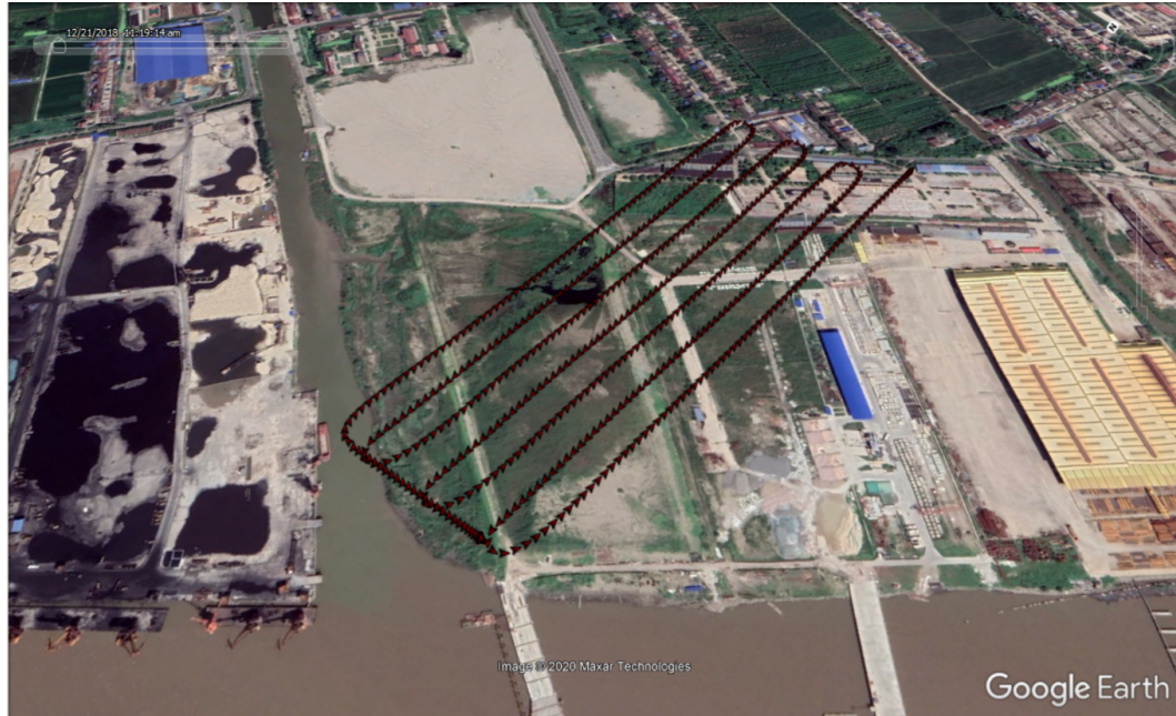
Figure 5.6: Graphical overlay of the flight path simulated by Acienna. The path included an initial rise to altitude and then has several switchbacks. This path is simulated based on a series of defined change rates and duration values. This map was obtained using Google Earth.
