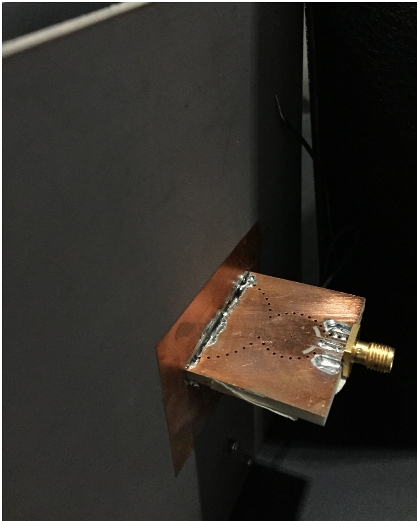
Figure 6.10: Back of the completed 125 mil filtenna.
