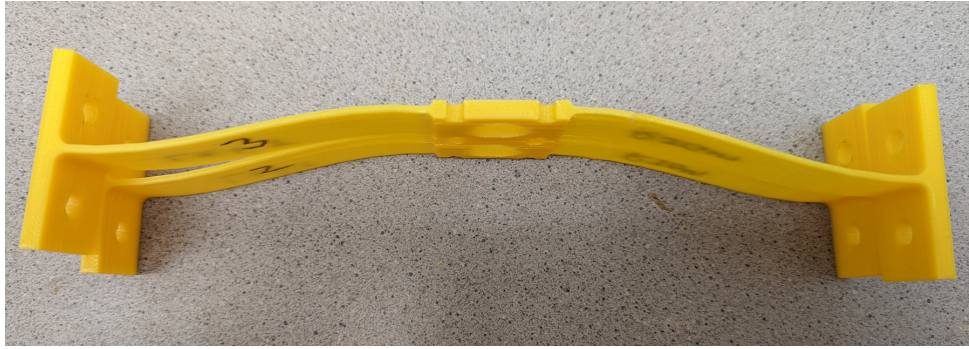
Figure 3.12: An example of the plastic deformation experienced by the beams following static testing. These beams are lined up at the center. Pictured are beams 2 (bottom) and 3 (top).
