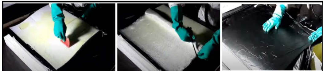
Figure 9: Method of applying fiberglass cloth with epoxy and curing airfoils. [2]
