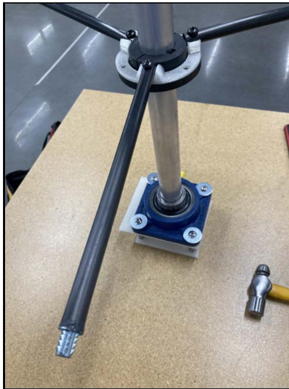
Figure 14: Carbon fiber strut bar, Strut-collar attachment, and Flanged Shaft Collar assembly as well as flanged bearing
