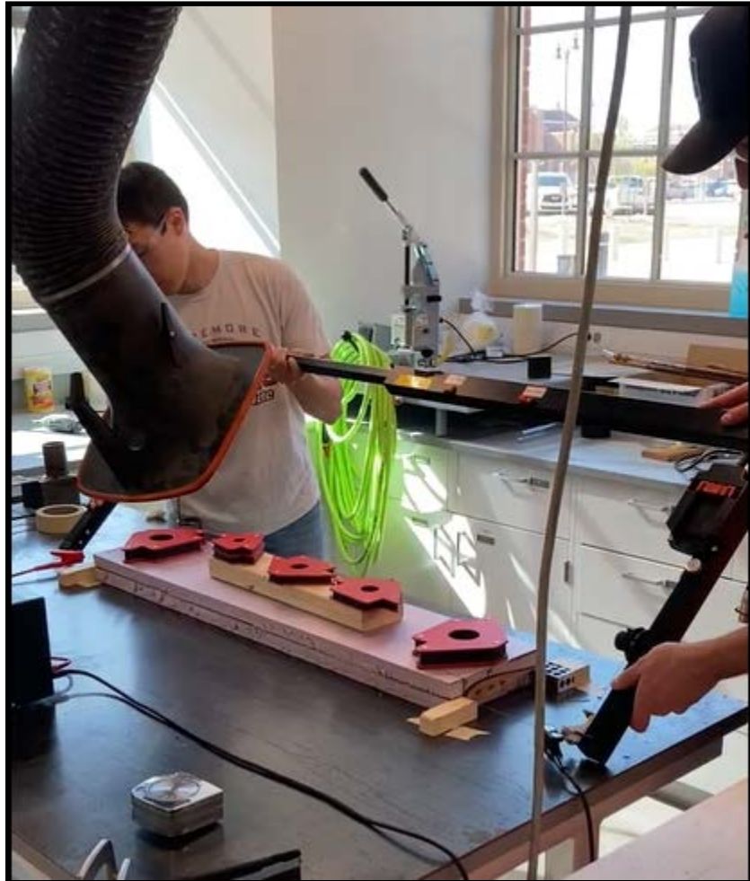
Figure 8: Using a hot wire bow unit to cut airfoils out of foam. [1]
