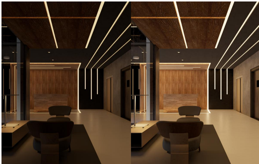
Figure 5 & 6 A Comparison Between Lux Level of 140 (left) and Lux Level of 538 (Right) by Using BIM Model Designed by Researcher
