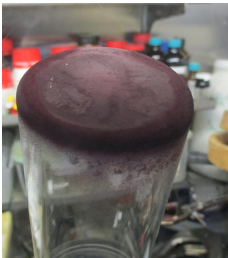
Figure 0.2: Tris[bis(trimethylsilyl)amido]uranium(III), \text{U}[\text{N}(\text{SiMe}_3)_2]_3 , deposited on sublimation apparatus. Sublimed by Stewart Younger-Mertz (Spring 2018).
