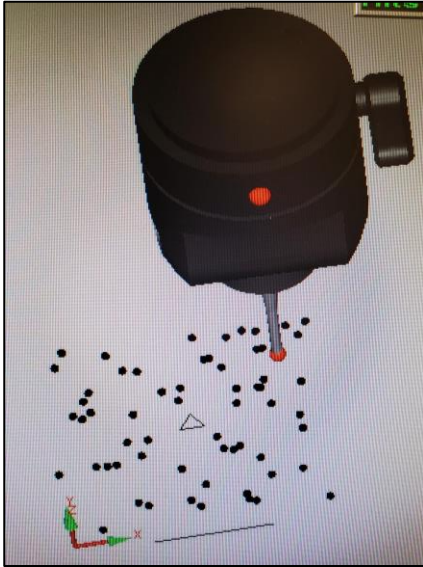
Figure 5. PC-DMIS virtual representation of the probe and the points on the surface of the part
