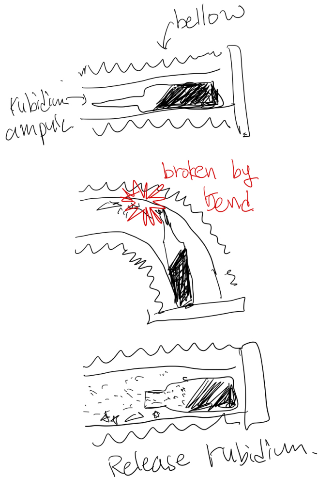
Figure A.3: Usage of the bellow to release rubidium into the high voltage chamber.
