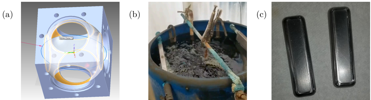
Figure 5.7: (a) Spherical area inside the chamber made with mechanical grinding with a CNC (Computer numerical control) machine, (b) electropolishing of the plates to remove a thin layer of material from the stainless plates, and (c) plates after mechanical and electropolishing of their surfaces.
