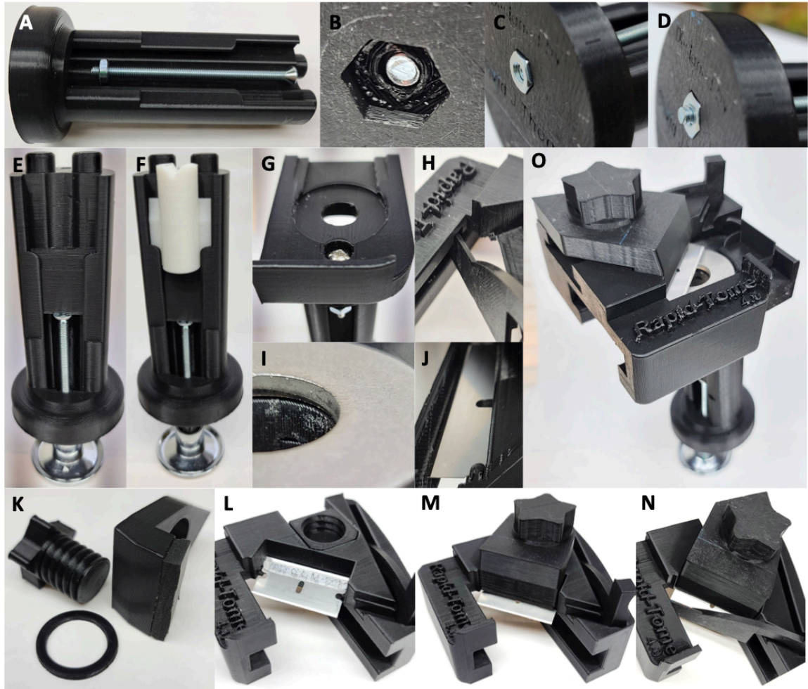
Figure 5.4. Assembly of the Rapid-Tome. (A-D) The advancement bolt is installed first. (E-G) The slider is placed within the grooves of the handle before the stage is attached. Optional longitudinal slider (white) is shown in (F) that can be stacked on top of a slider. (H-J) The washer and blade guard are attached. The blade clamp (K) is crucial and holds the blade in place (L-N). Sliding the sled into place over the stage against the inclined washer flexes the blade and ensures a flat cut is made. All plastic parts are 3-D printed with PLA.
