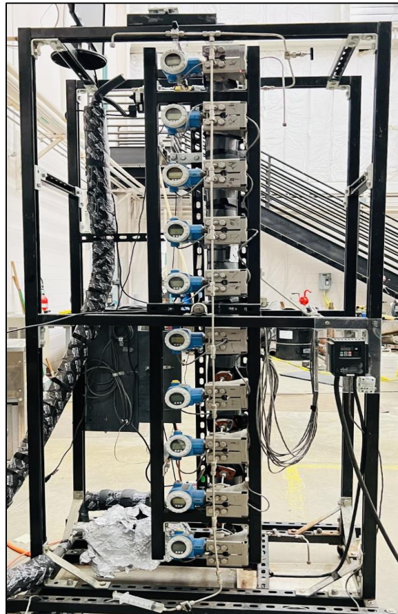
Figure 3.3: Experimental setup of vertical drainage test section
