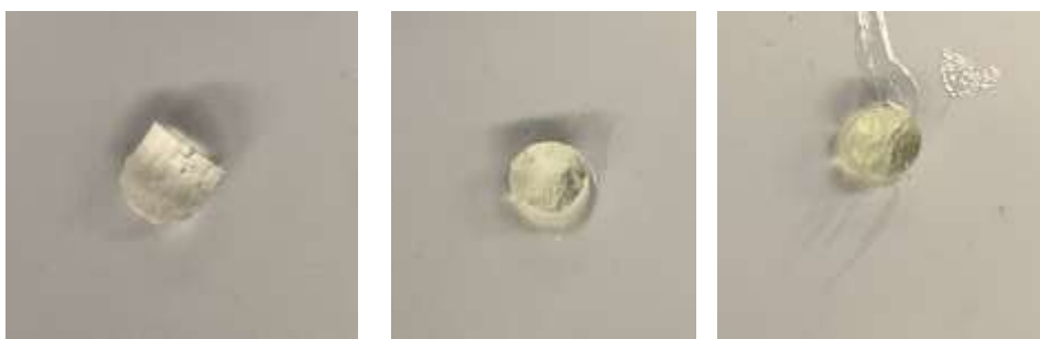
Figure 4-IV: Images showing the coloring of PMOEP after polymerization at 50 °C with native pH (left), pH 1 (center) and pH 1.5 (right).
