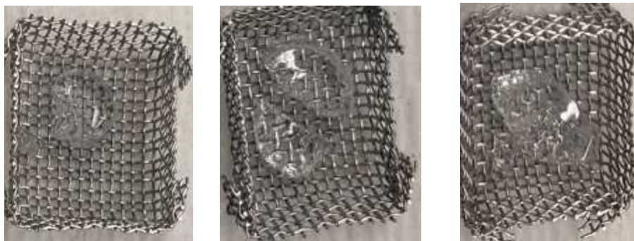
Figure 4-V: PMOEP polymerized at 50 °C with its native pH (left), pH 1 (center) and pH 1.5 (right) showing fracturing became more severe as pH increased.
