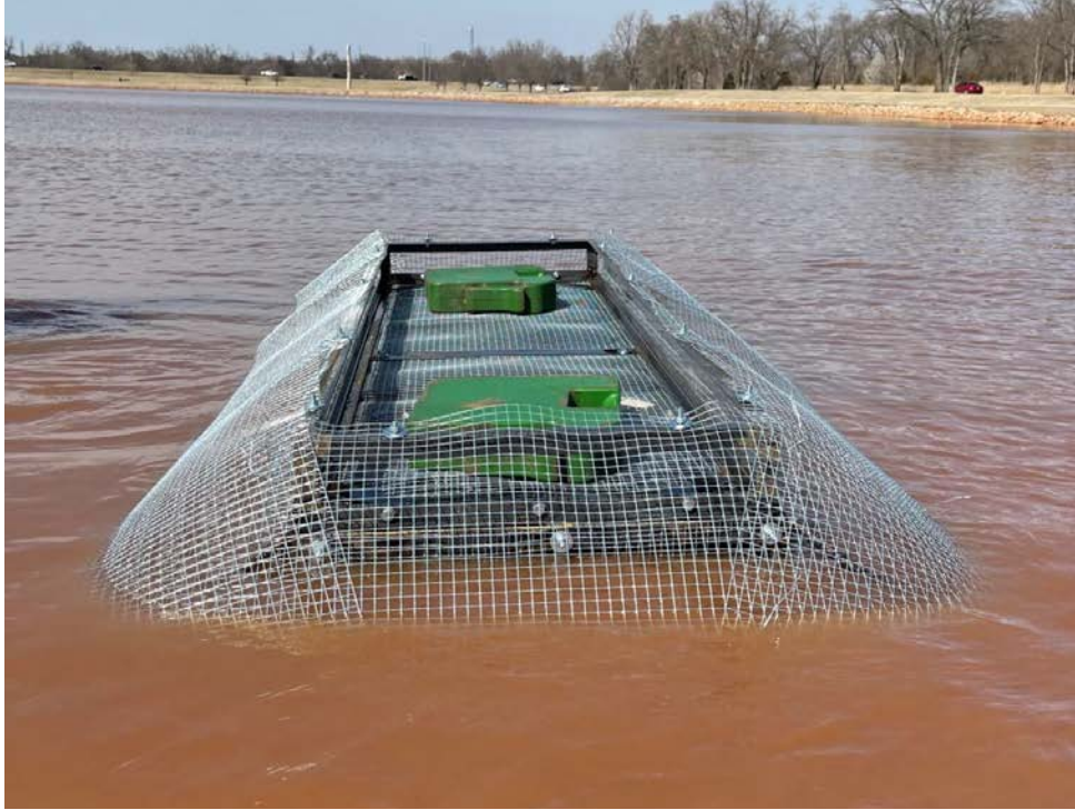
Figure 38. Frame Float Test 64 kg
