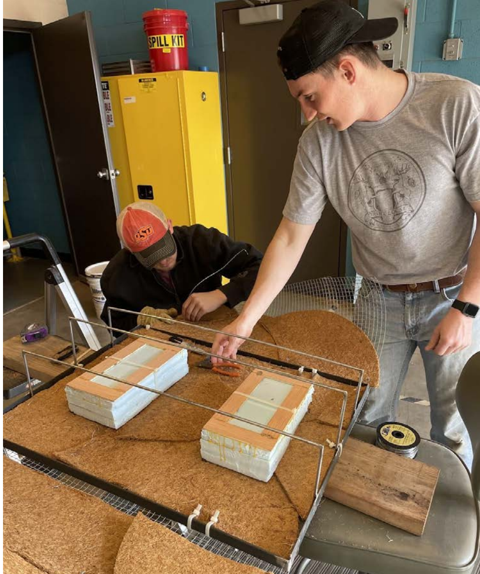
Figure 18. Adding Media and Floatation to the Quarter Scale Prototype
