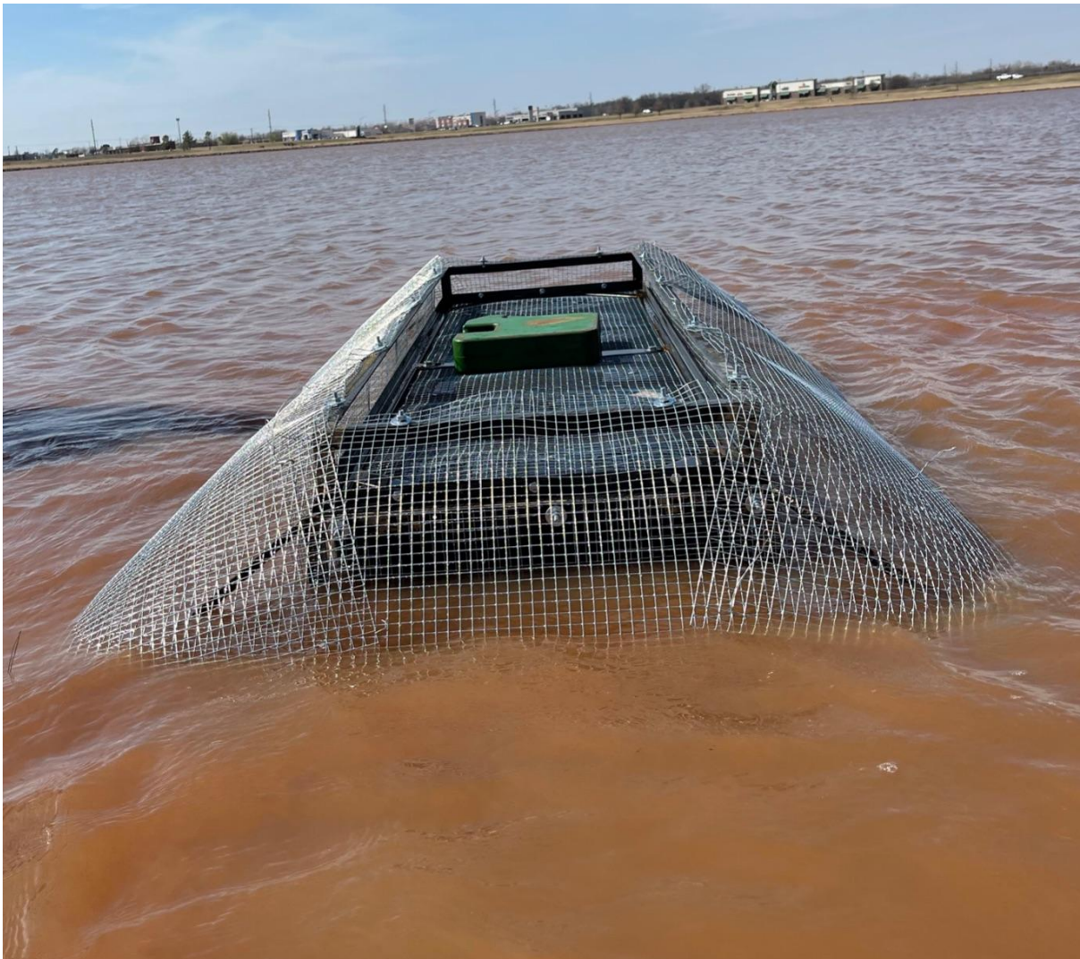
Figure 37. Frame Float Test 32 kg
