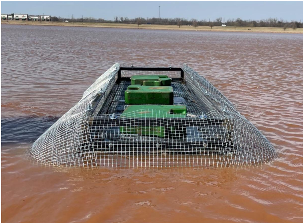
Figure 39. Frame Float Test 96 kg
