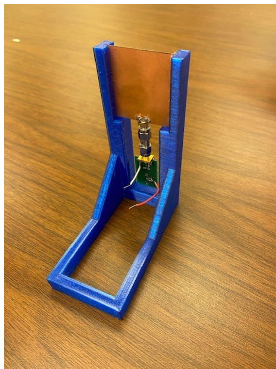
Figure 24: Rectifier PCB and Antenna Mounted on Stand
