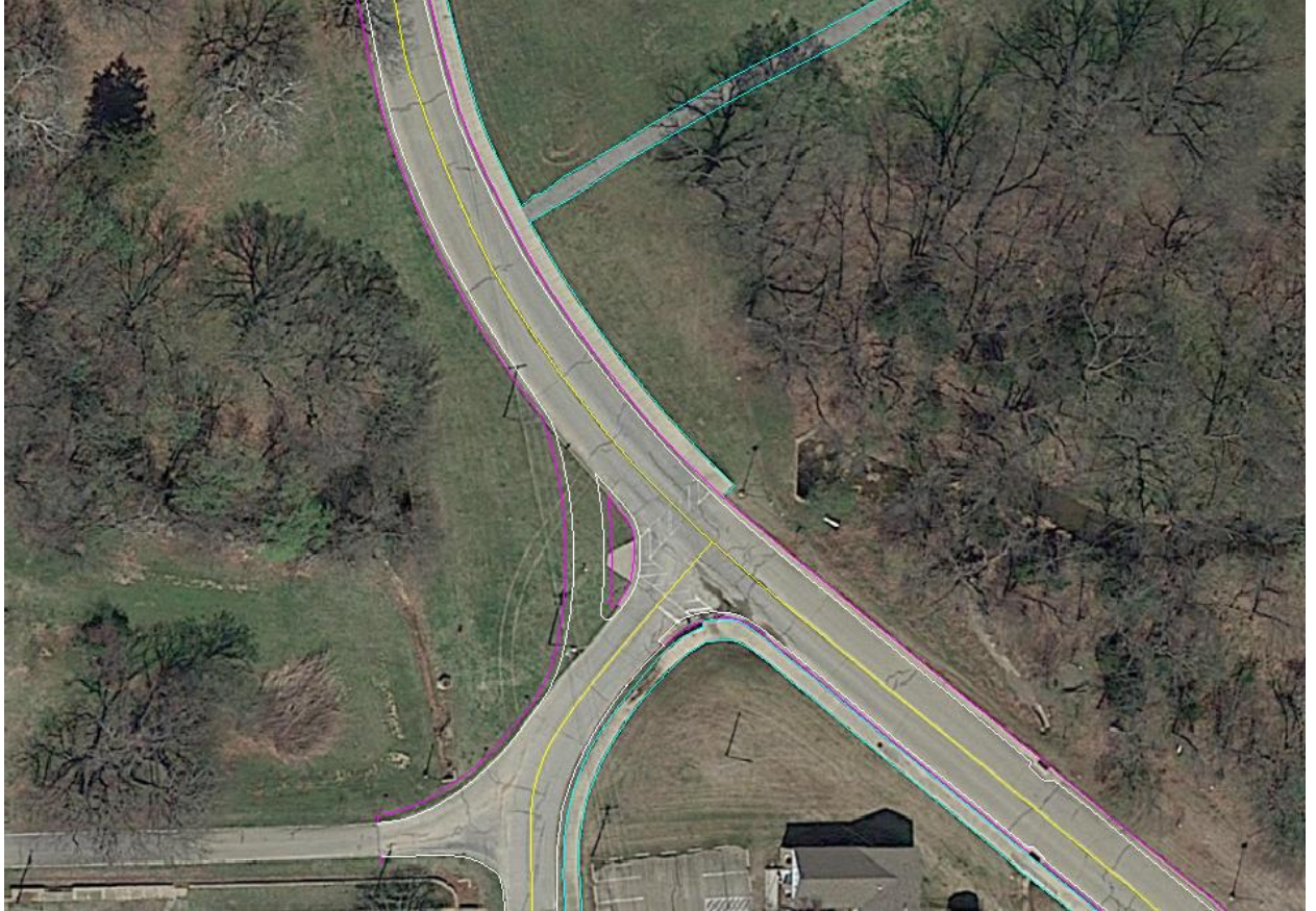
Figure 11: Right-turn slip lane design at the intersection
