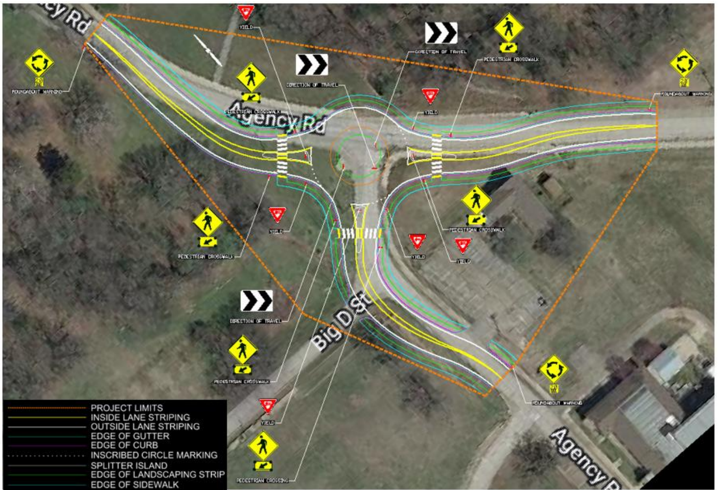
Figure 33: Roundabout design containing signage in MicroStation
