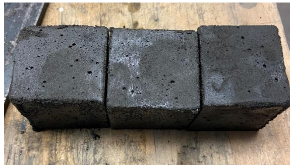
Figure 3.2 Overdosed Cube Specimens Demolded
