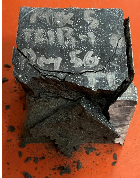
Figure 4.6 Typical 56 Day Break Failure Morphology
