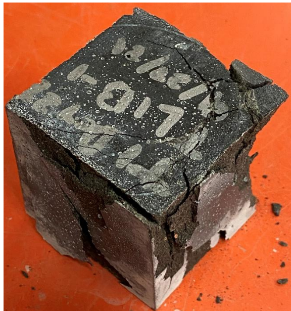
Figure 4.5 Typical 28 Day Break Failure Morphology
