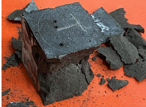
Figure 4.4 Typical 14 Day Break Failure Morphology
