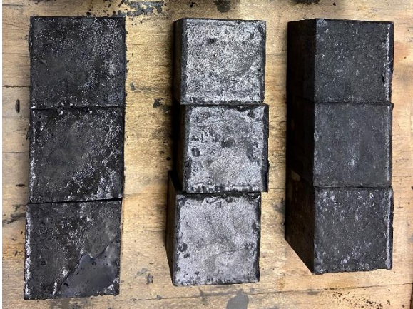
Figure 3.4 Mix 12 Cube Specimens Demolded
