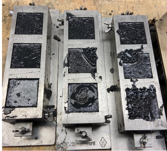
Figure 3.1 Overdosed Cube Specimens in Molds
