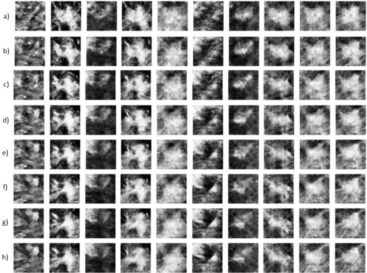
Figure 4-2: Generated images at a) 25,000 b) 50,000 c) 75,000 d) 100,000 e) 125,000 f) 150,000 g) 175,000 h) 200,000 epochs. The FID scores are a) 52.36 b) 53.53 c) 52.53 d) 52.59 e) 51.50 f) 51.07 g) 51.74 h) 56.79 accordingly.
