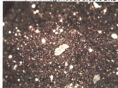
Bitumen Homogeneous 0.65% BRo
