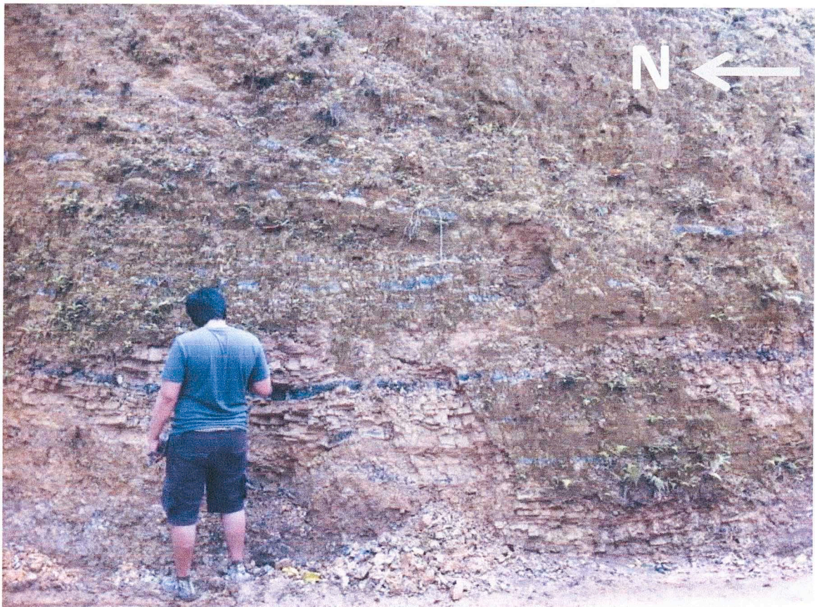
Figure 16. Bitumen layers between cherts, claystone and siliceous mudstone beds of the Pujamana member, in OUTCROP B.
