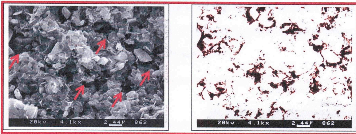
Figure 87. SEM analysis of sample P2M1 corresponding to micritic Packstone. Image on the right is at 4,100X of magnification and shows interparticle porosity indicated by red arrows. The image on the right shows the total associated porosity by highlighting the pore spaces. TOC% = 1.51%.
