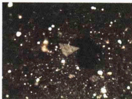
CAR M-2. Bitumen granular 0.45% BRo CAR M-2. Bitumen granular 0.43% BRo
