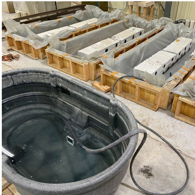
Figure 5-2: Saline solution transferring to specimen baths
