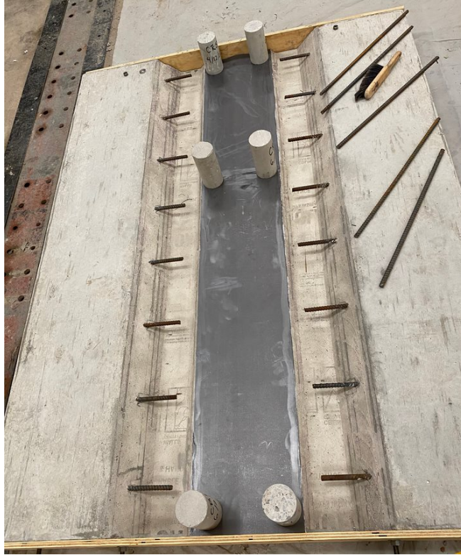
Figure 3-19: Connection preparation with sheet gasket installed
