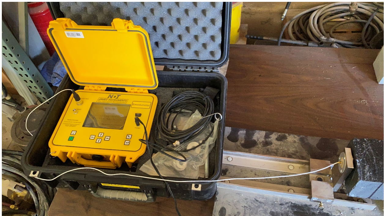
Figure 4-11: Emodimeter with accelerometer connected (white wire)
