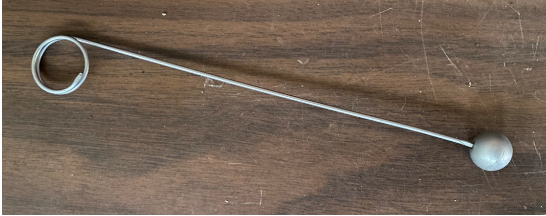
Figure 4-10: Steel impactor used to collect frequency readings
