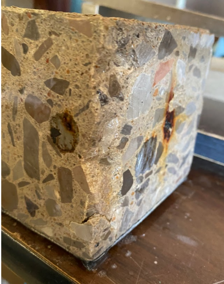
Figure 4-19: Chipped edges of specimen AA2-L
