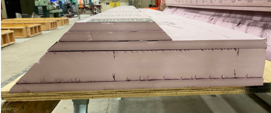
Figure 3-7: Connection cavity foam insert cross-section
