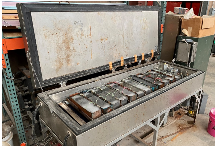
Figure 4-7: Freeze-thaw specimens thawing in cabinet
