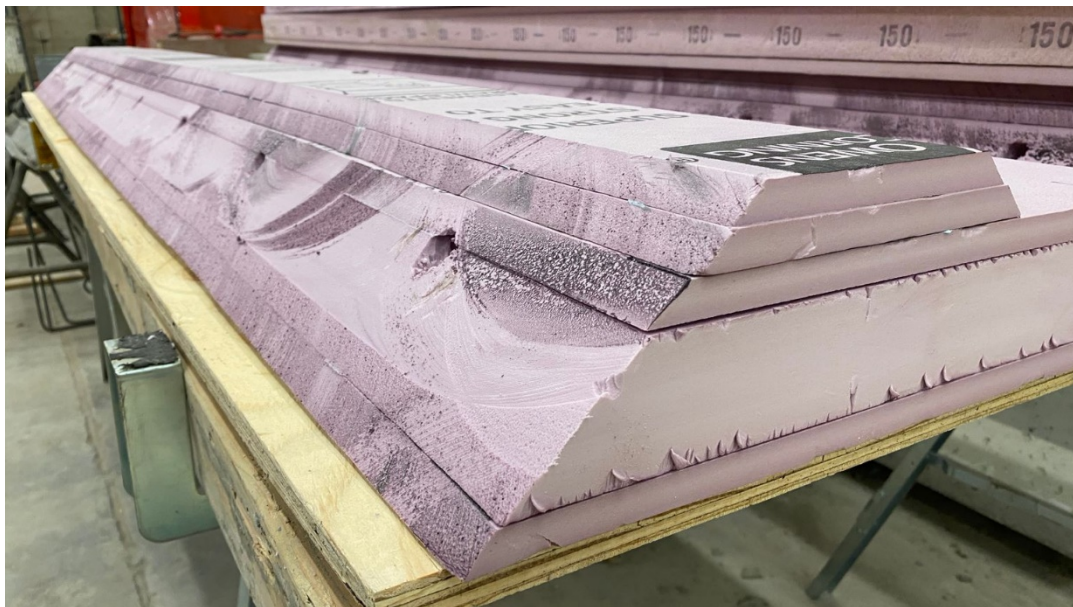
Figure 3-8: Foam insert with drilled holes for rebar
