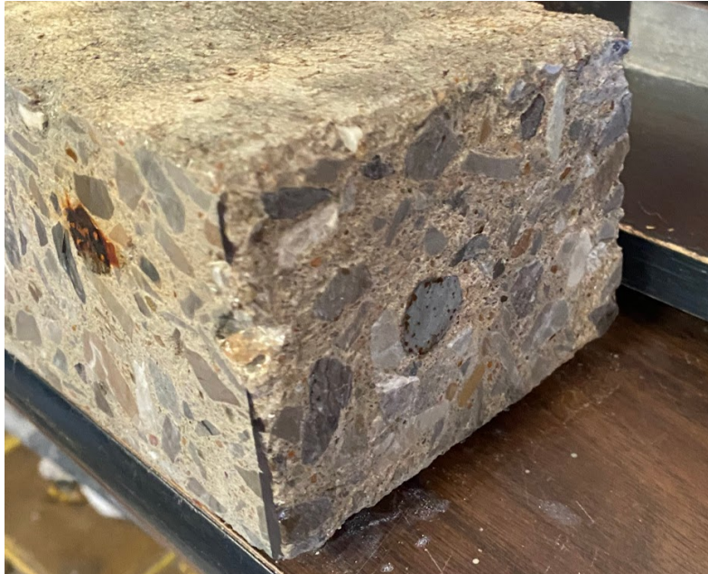
Figure 4-18: Chipped edges, face of specimen AA3-N
