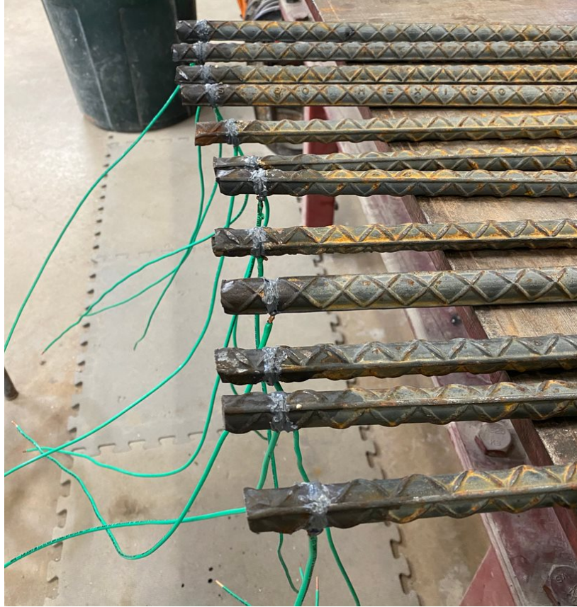
Figure 3-20: #5 rebar soldered with copper wire
