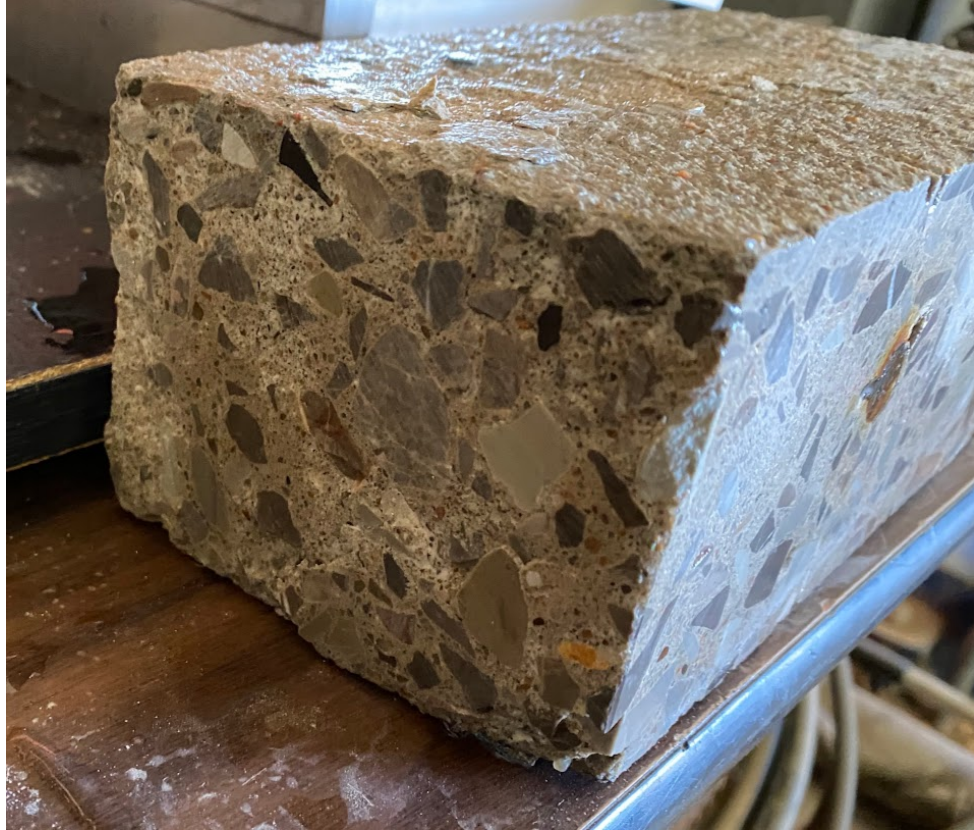
Figure 4-20: Chipped edges, face of specimen AA3-L
