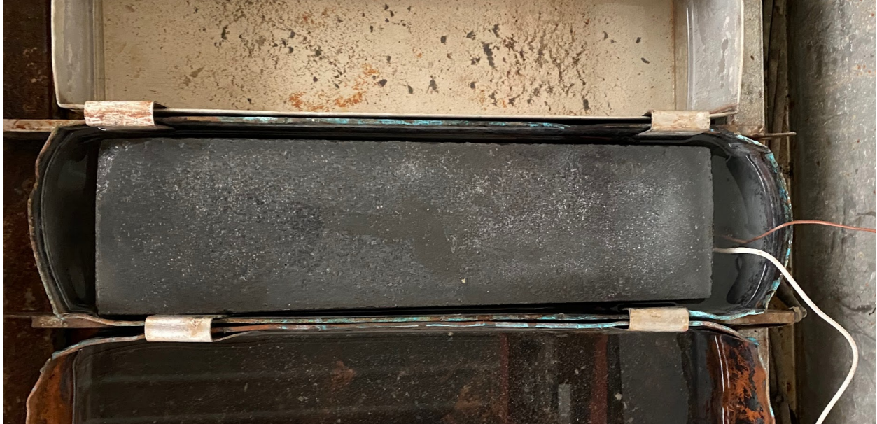
Figure 4-6: Control specimen in freeze-thaw tray
