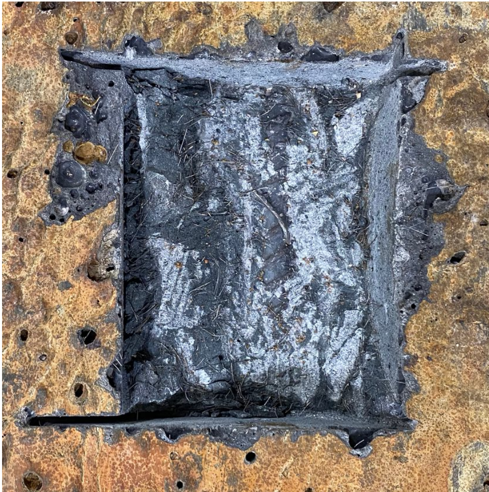
Figure 5-16: CU-L observed rebar A, 37 days tested
