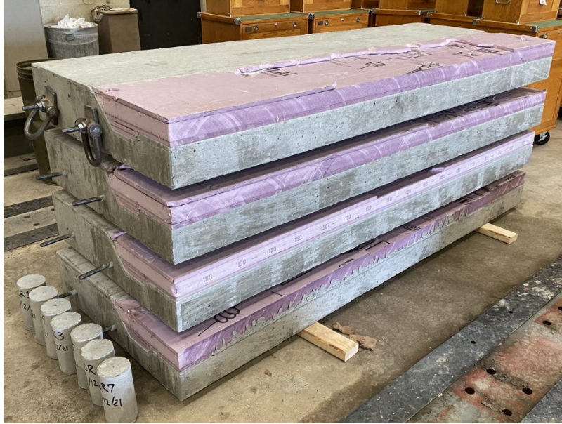
Figure 3-16: Slab sections after demolding, flipping
