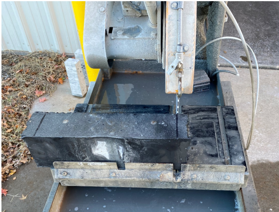
Figure 4-3: Cutting freeze-thaw specimen to length
