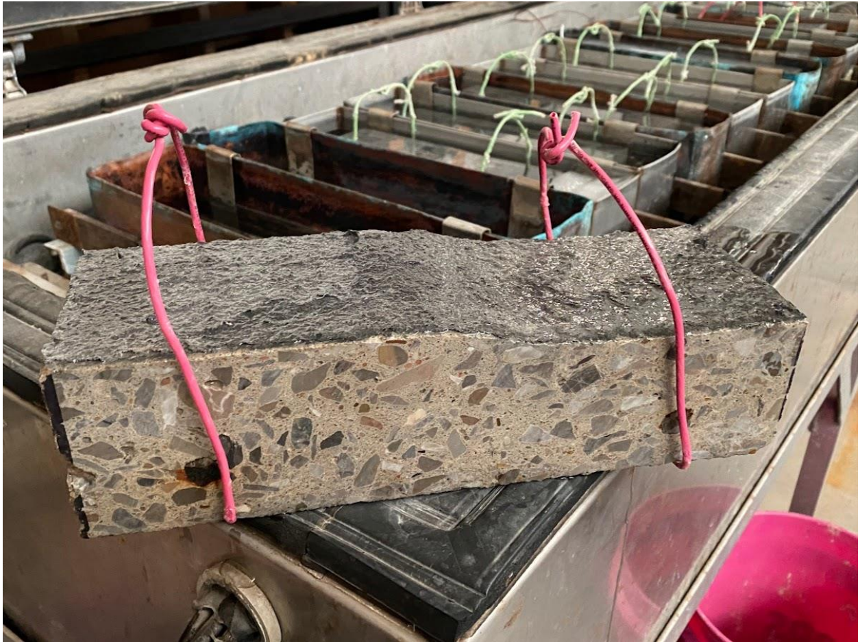
Figure 4-8: Standard orientation of specimen placed in freeze-thaw tray
