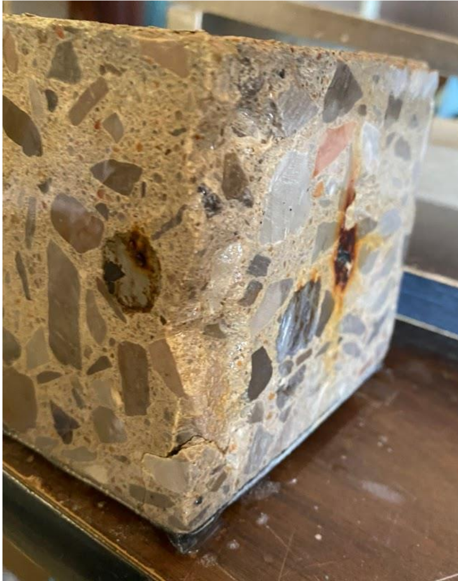
Figure 4-19: Chipped edges of specimen AA2-L
