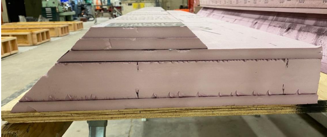
Figure 3-7: Connection cavity foam insert cross-section
