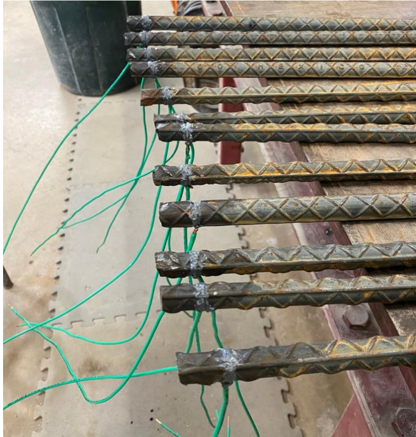
Figure 3-20: #5 rebar soldered with copper wire
