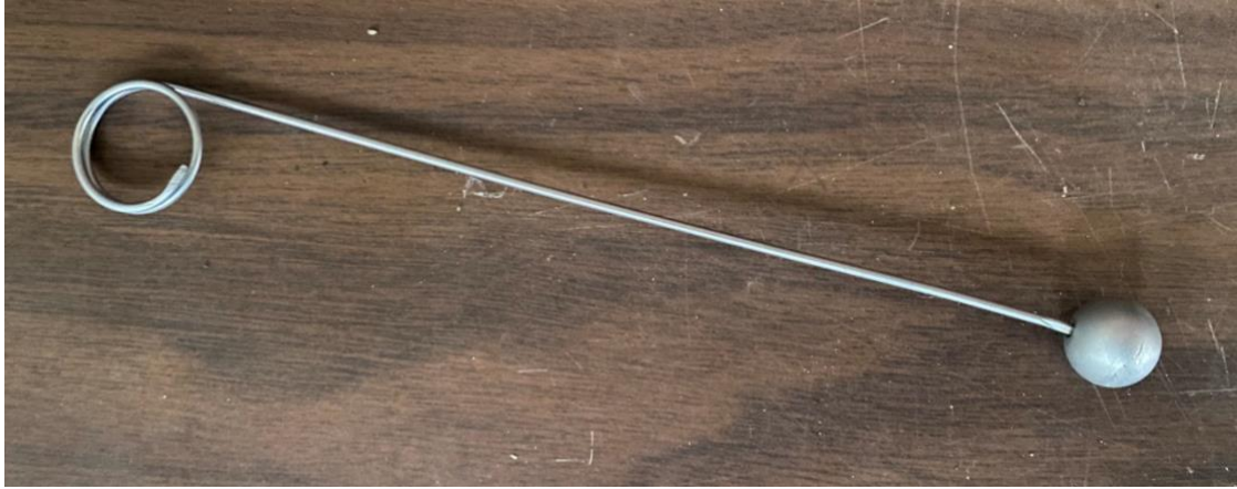
Figure 4-10: Steel impactor used to collect frequency readings
