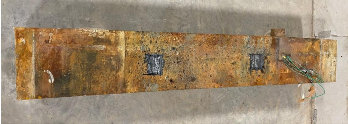
Figure 5-15: Surface of CU-L after 37 days of testing, windows cut
