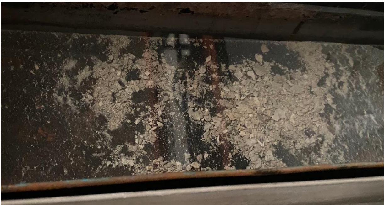
Figure 4-16: Concrete residue in tray after removal of specimen AA2-L
