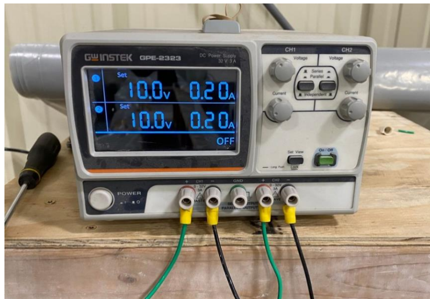
Figure 5-3: DC power supply with test settings
