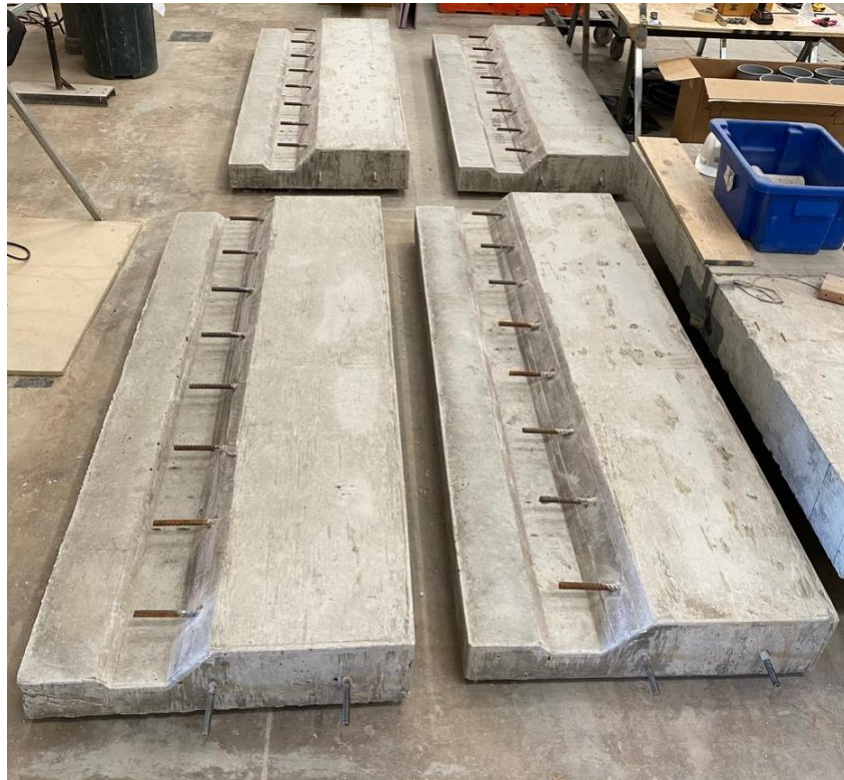
Figure 3-17: Slab sections with foam removed
