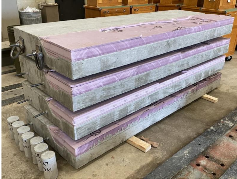
Figure 3-16: Slab sections after demolding, flipping
