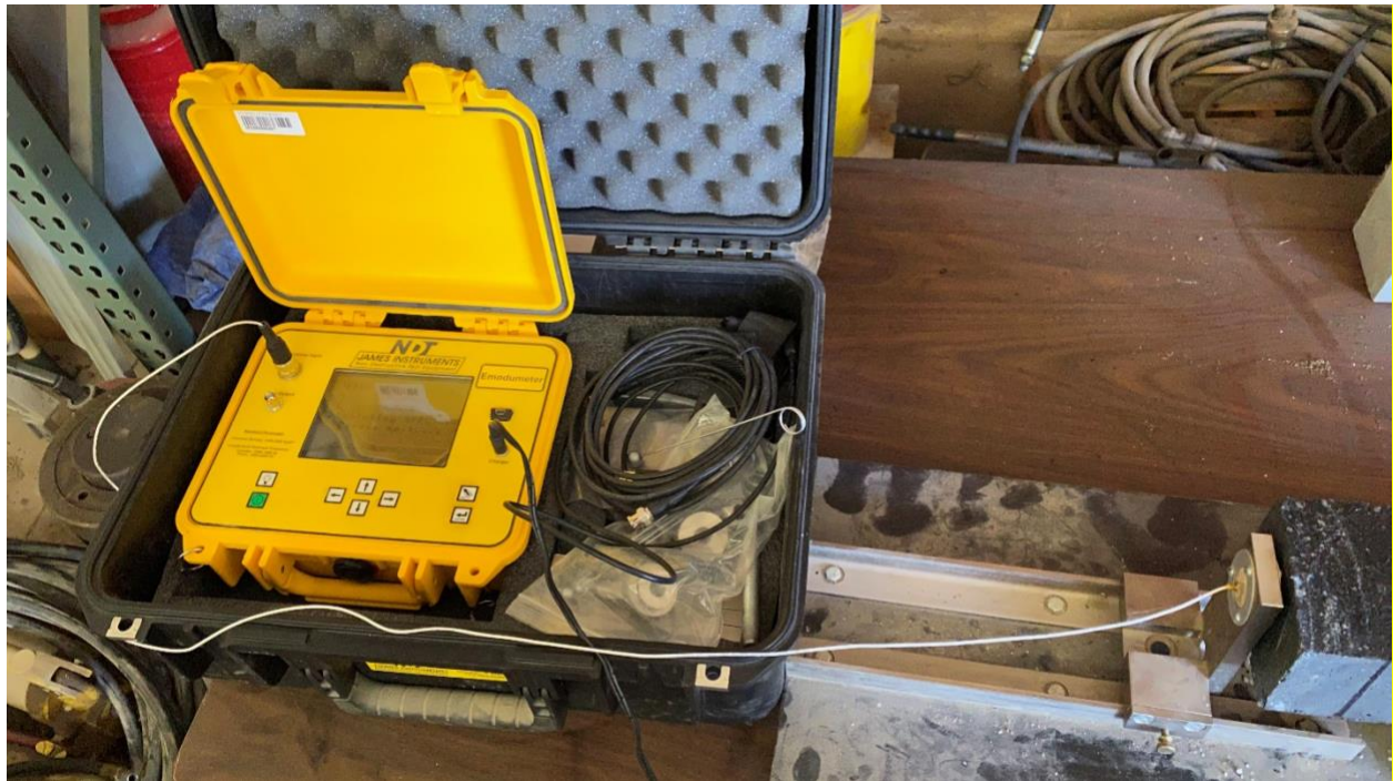
Figure 4-11: Emodometer with accelerometer connected (white wire)
