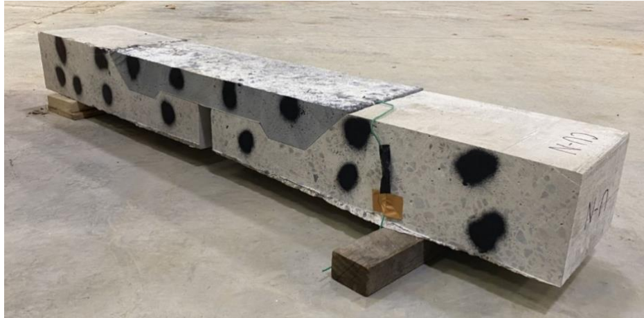
Figure 5-1: Corrosion specimen CU-N with sealant applied to exposed rebar ends
