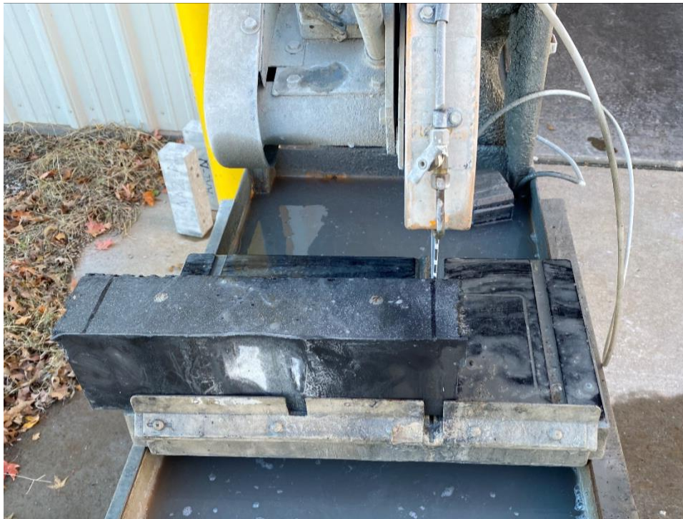
Figure 4-3: Cutting freeze-thaw specimen to length
