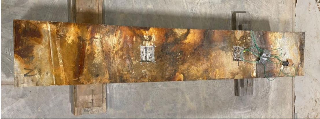
Figure 5-11: Surface of CAA-N after 37 days of testing, windows cut
