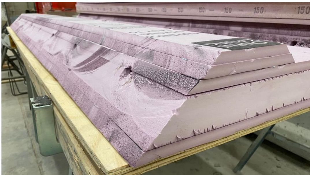
Figure 3-8: Foam insert with drilled holes for rebar
