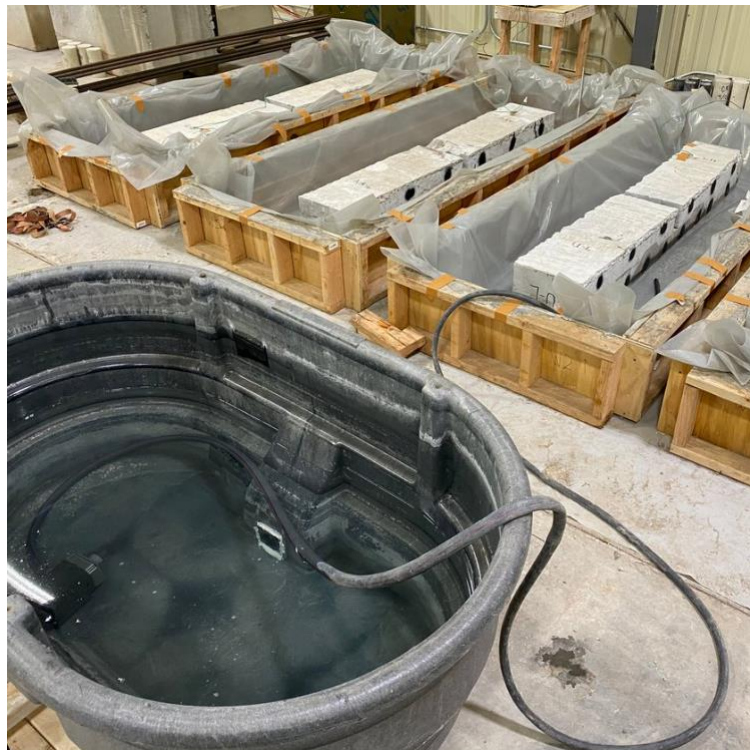
Figure 5-2: Saline solution transferring to specimen baths
