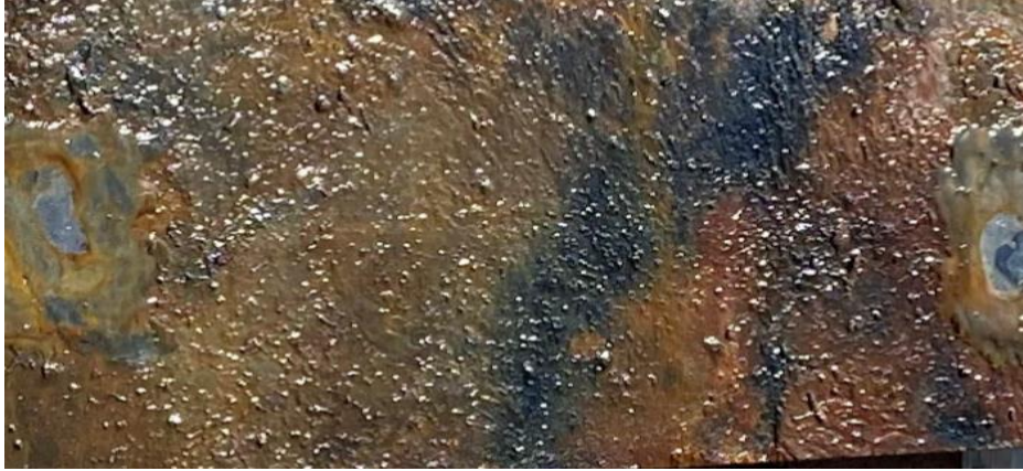
Figure 5-31: Surface of specimen CU-N after 65 days of corrosion testing
