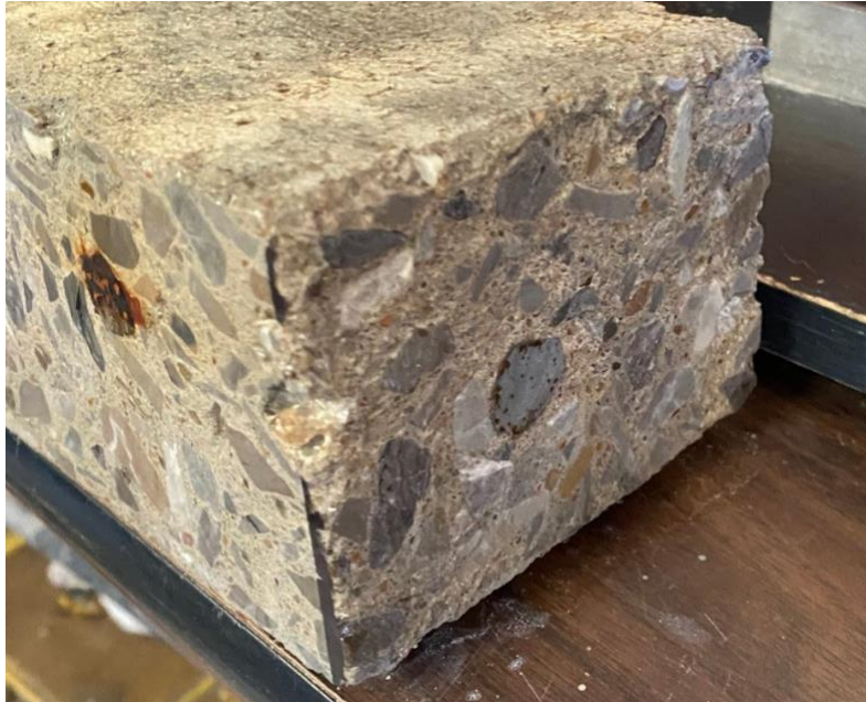
Figure 4-18: Chipped edges, face of specimen AA3-N
