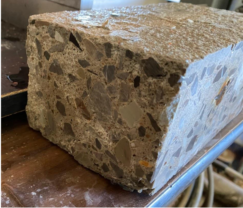
Figure 4-20: Chipped edges, face of specimen AA3-L
