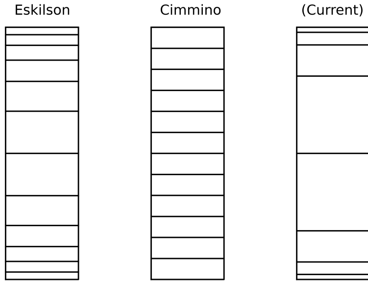
Figure 4.3: Eskilson’s 12 segment discretization scheme, Cimmino’s uniform discretization and the current segment ratio discretization using an end length ratio of 0.02 with 8 segments.
