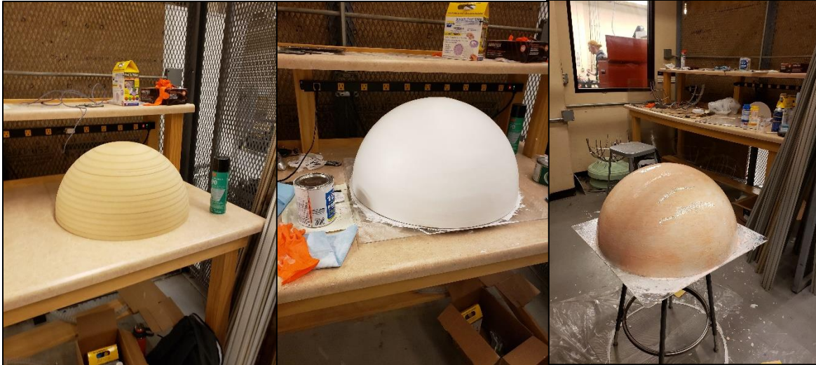
Figure 16: (Left) Creation of MFD Mold, (Center) Preparation for Casting, (Right) Casting Shell
