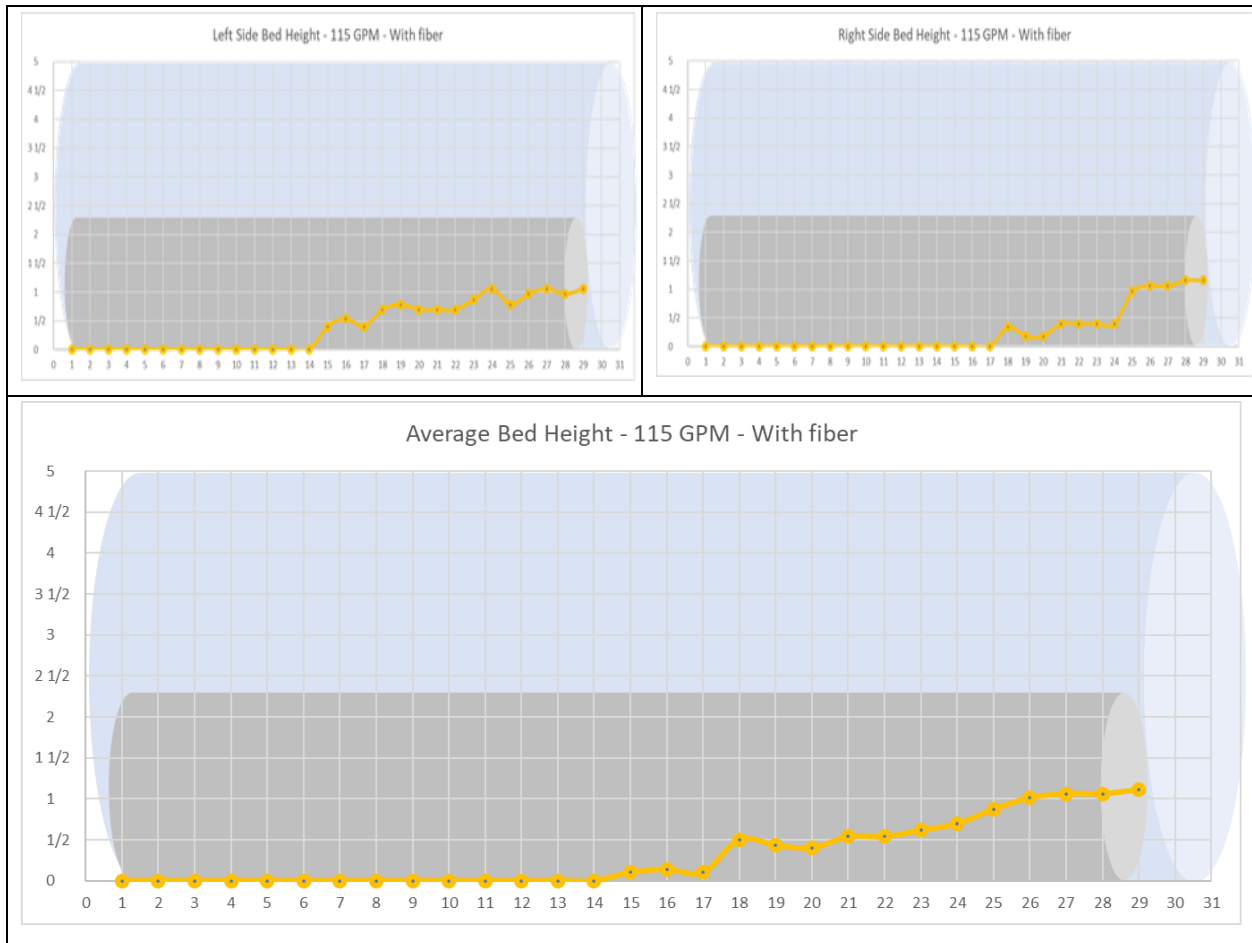
Figure A.28 Fibrous cleaning fluid left-side, right-side, and average bed profiles (115 GPM, 50 RPM)
