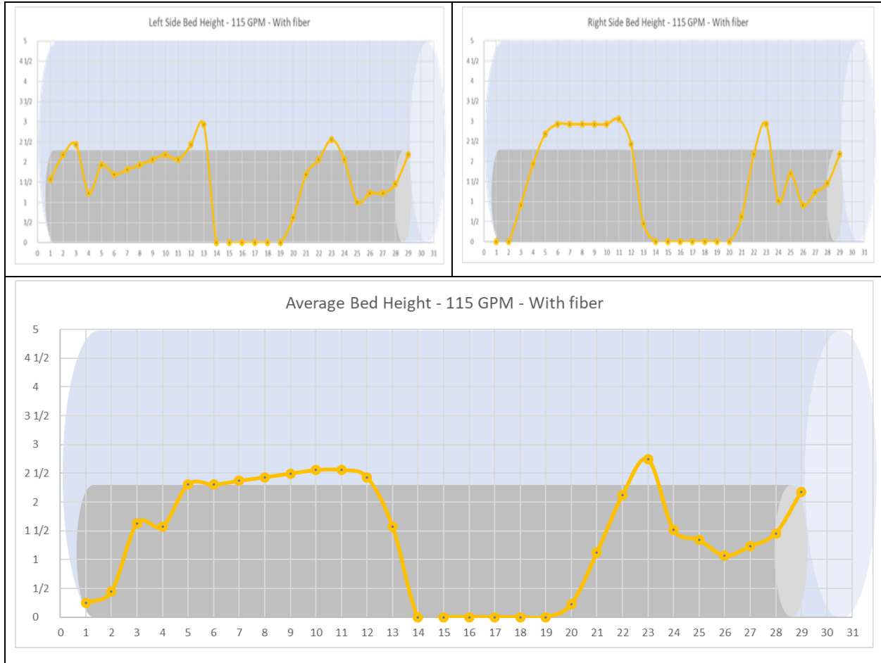
Figure 6.4 Fibrous fluid left-side, right-side, and average bed profiles (115 GPM, 0 RPM)
