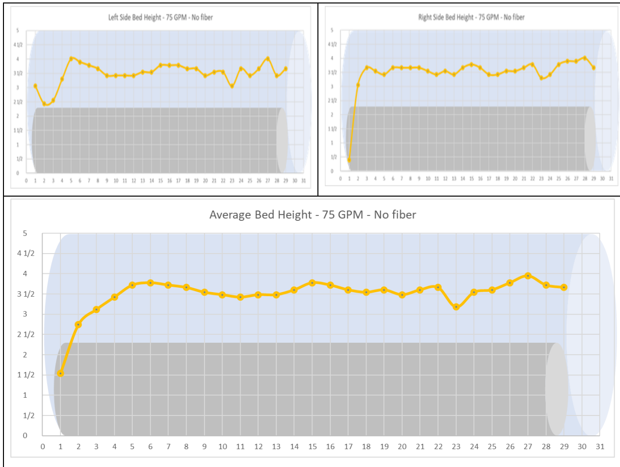
Figure A.10 Base cleaning fluid left-side, right-side, and average bed profiles (75 GPM, 0 RPM)
