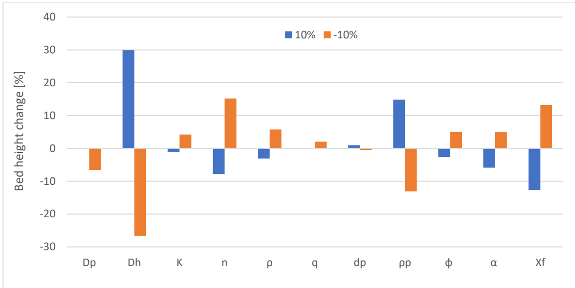
Figure 6.15 Sensitivity plot for equilibrium bed height ( q=155 GPM)
