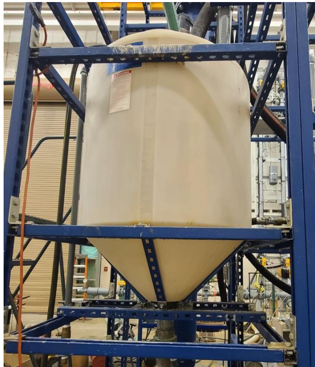
Figure 4.2 Mixing tank of the flow loop
