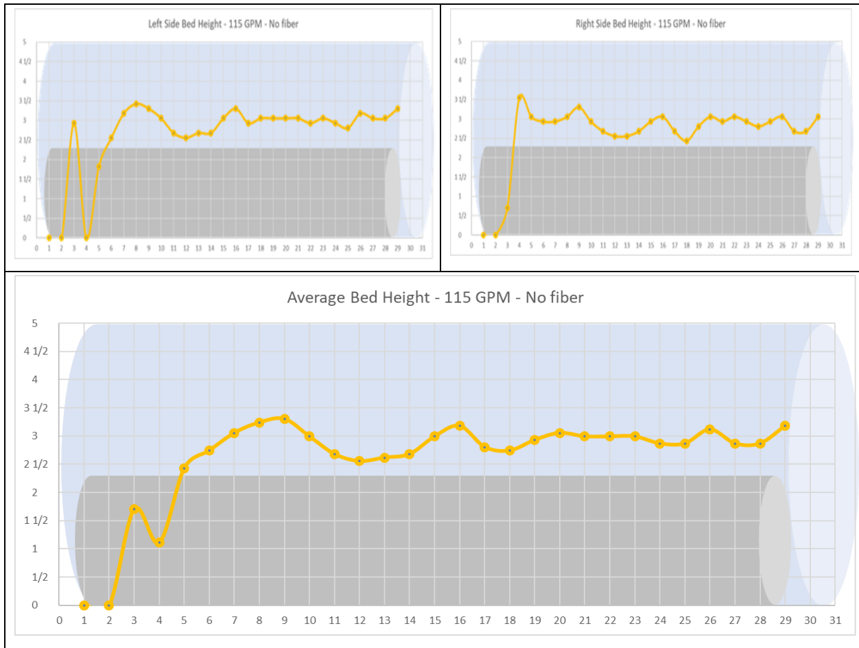
Figure A.11 Base cleaning fluid left-side, right-side, and average bed profiles (115 GPM, 0 RPM)
