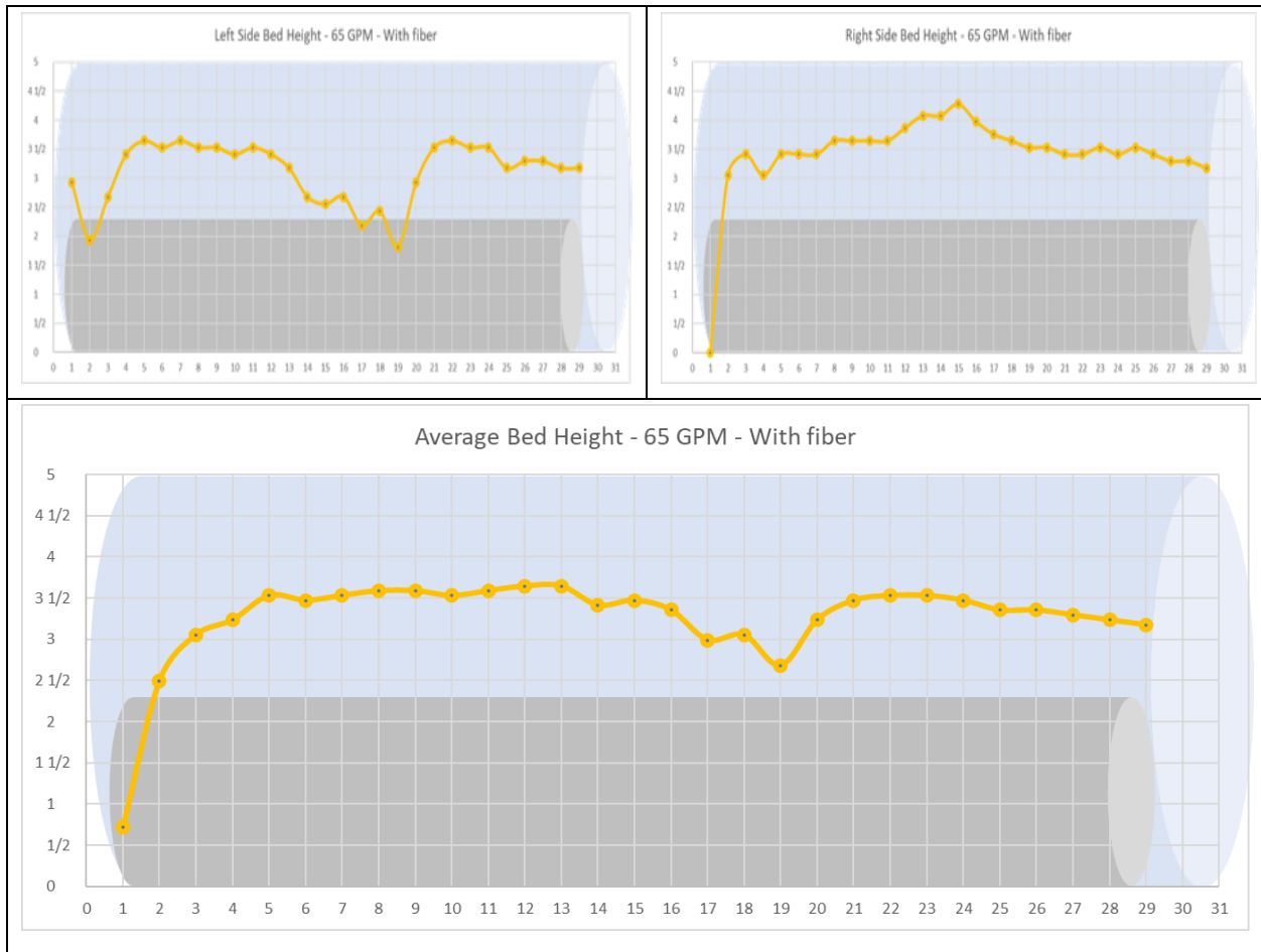
Figure 6.5 Fibrous fluid left-side, right-side, and average bed profiles (65 GPM, 0 RPM)
