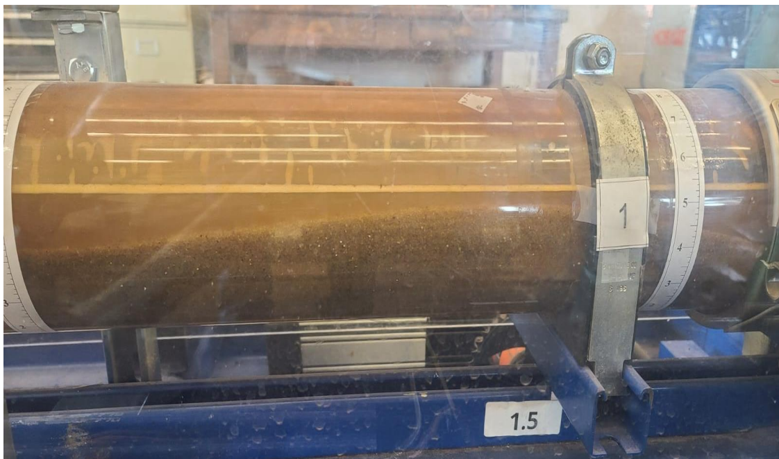
Figure 4.5 Solids depositing on the horizontal annular test section
