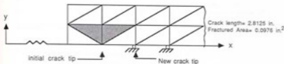
(b) Boundary Conditions after first element fractured and before second element fractured
