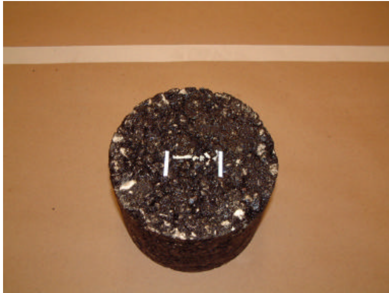
Figure 8-3: Prepared sample ready for crushing
