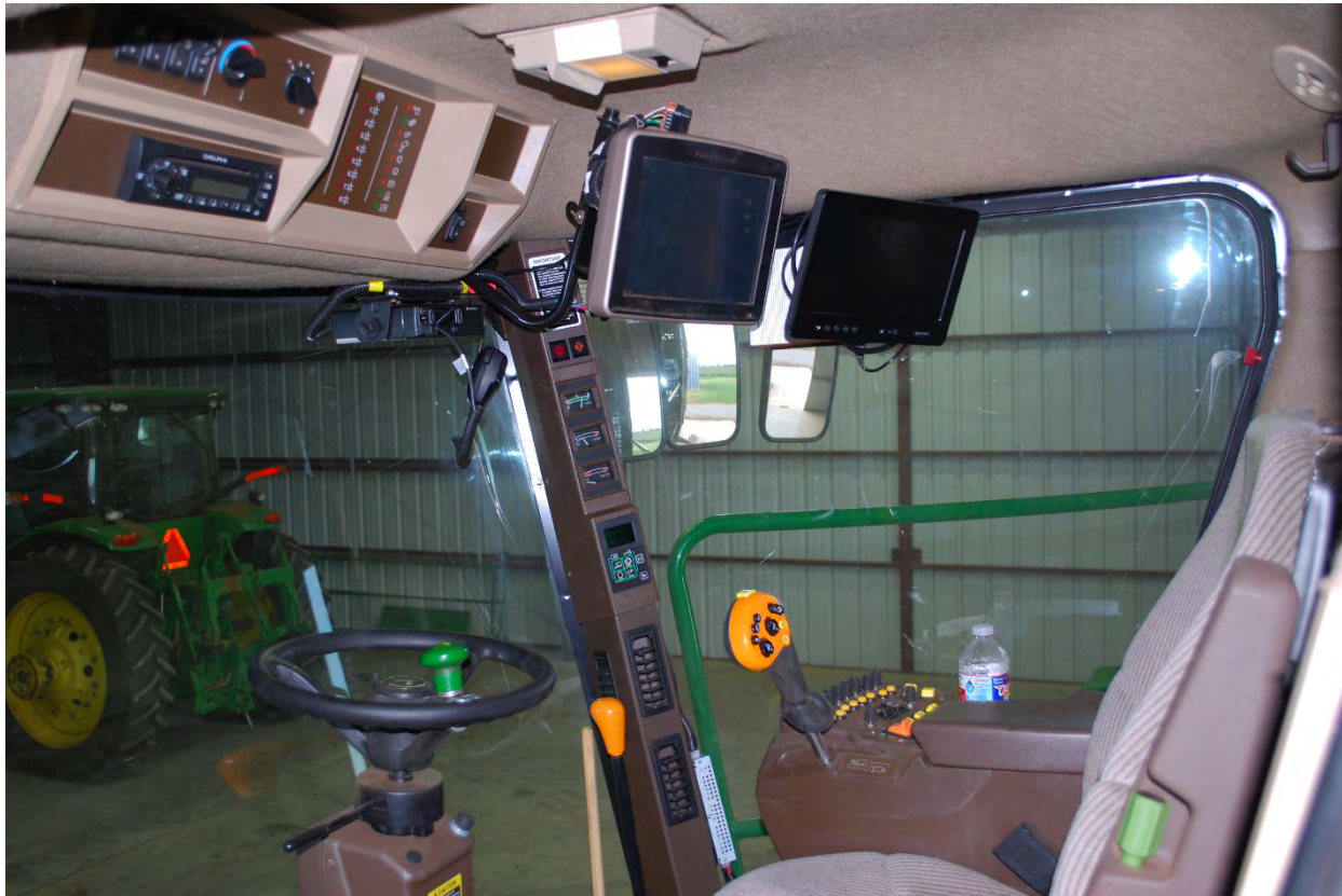
Figure 5. Weighing system touch screen display (right) and John Deere 2630 yield monitor display mounted in the cab of a John Deere 7460 cotton stripper.
