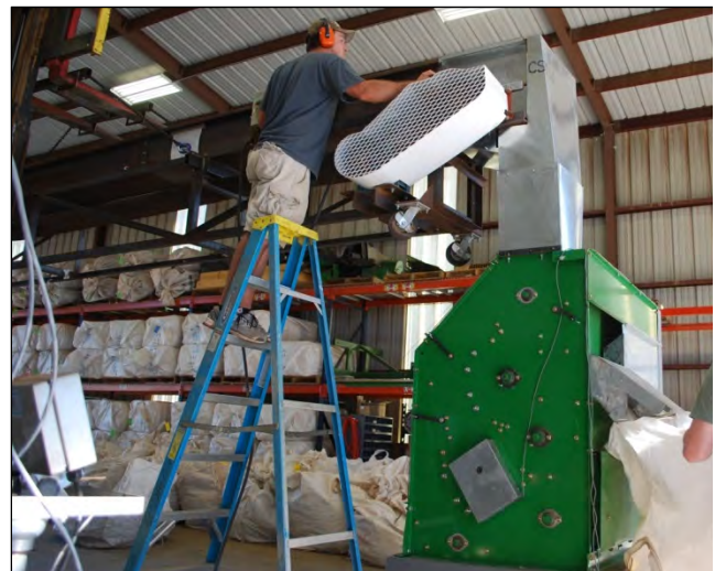
Figure 4. The flow rate simulator used to control the material being conveyed into the laboratory field cleaner.
