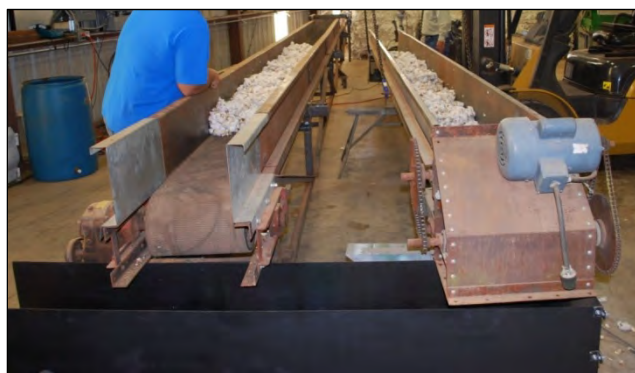
Figure 1. The two flow rate simulators used to control the material being conveyed onto the wire belt conveyor.
