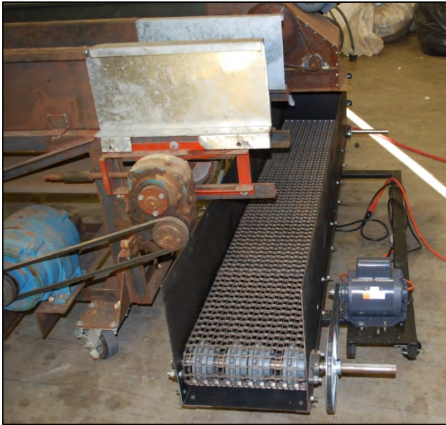
Figure 2. The wire belt conveyor used as a comparison to the cross auger.
