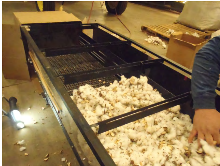
Figure 3. The guide marks on the divider were used to ensure the bur cotton bat was placed at the appropriate depth and can be seen on the right to the far end of the wire belt conveyor.
