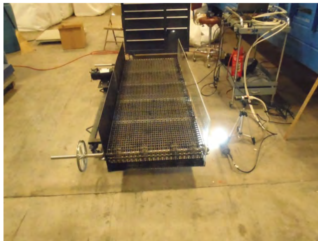
Figure 4. The high speed camera and the belt conveyor with the plexi-glass side installed.
