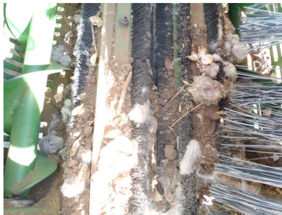
Figure 5. The excessive dirt collected by the stripper rolls.
