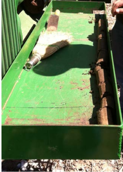
Figure 2. Soil core in tray used for dividing samples into depths.
