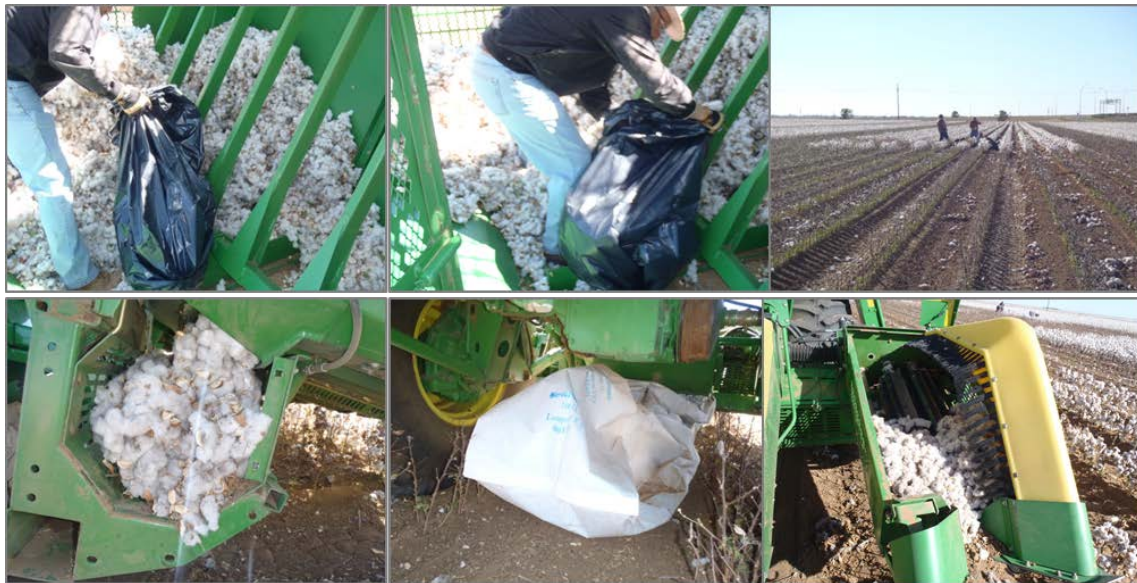
Figure 1. Clockwise from top left to bottom left: Before Field Cleaner, After Field Cleaner, Hand Harvested, After Brush Rolls, After Cross Auger, and After Row Unit.
