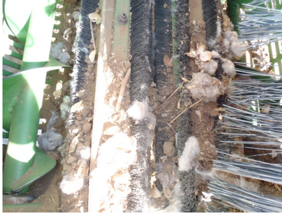
Figure 2. Excessive dirt in the stripper rolls.
