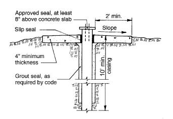
Figure 1. Recommended construction for water wells to protect the ground water supply from contamination.
