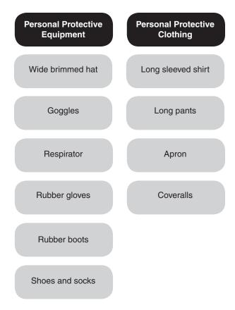
Figure 1. List of personal protective equipment and personal protective clothing.
