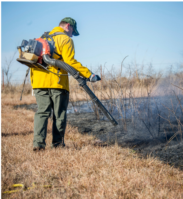
Leaf blowers can be used for many different tasks on prescribed burns. One of the most common uses for a leaf blower is to clear a line down to bare mineral soil; thus creating a firebreak. When in light fuels or working along the backfire/ flankfire, leaf blowers can be used to suppress fire. Leaf blowers are extremely effective on mopping up mulch piles, cow chips and small brush piles. (Photo courtesy T. Johnson)
