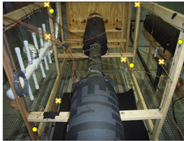
✱ Thermocouples ● Relative humidity sensors
