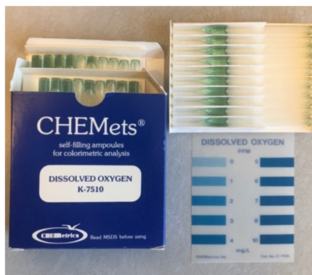
Figure 1. A relatively inexpensive chemical test kit for dissolved oxygen concentration. The ampule neck is snapped, and water is drawn up into it. A simple color comparison indicates the concentration of oxygen.
