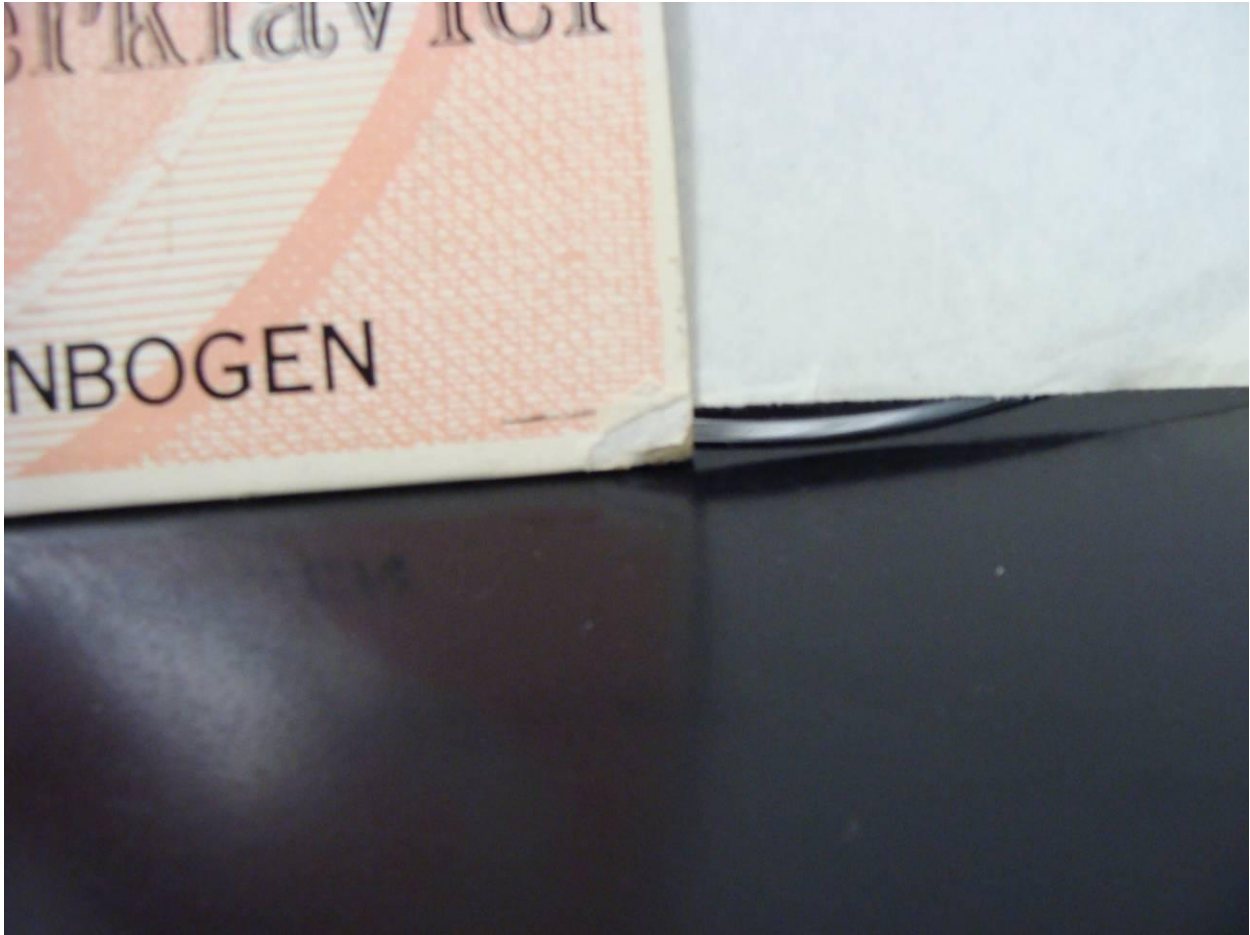
Figure 14: Acidic paper sleeve splitting at the bottom
