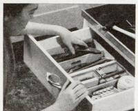
• Tool Kit. Minor mends save major -so keep a few tools handy. A kit with hammer, screw driver, pliers, nails, screws and tacks will be needed in a good-care program.
