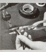
Mending Lamp Cord. Cut off worn cord. Loosen screws in plug and unfasten wires. Remove one and one half inches of outside cord covering—if braided wrap with string to stop raveling. Remove insulation from two inside wires for an inch from ends. Scrape wires bright but don't cut. Twist each wire. Insert cord through back of plug. Bring each wire around outside of one prong, wind bare portion around one screw and tighten screw. Bare wires must not touch each other.
