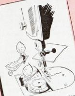
• Keep your machine clean. Excess oil catches dust wipe it off. Lint if left undisturbed packs around the bobbin and feed, clogging the machine, so wipe it out or remove it with a toothpick or darning needle.
