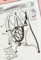
• Is yours a treadle machine? Then watch the belt. If it's too tight the machine runs hard and the belt wears out; if too loose it slips and half your effort is wasted. Shorten the belt a bit when it becomes too loose.
