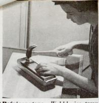
overwork refrigerators and prolong freezing. To flatten insert a block and pound. Frost-covered coils run motors overtime, defrost regularly. Oil and clean as directed. Hands off door gaskets-oil ruins rubber.
