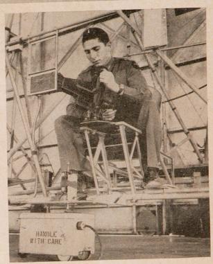
2. In high chair, simulating plane, cadet learns to train bombsight on moving electric target.
