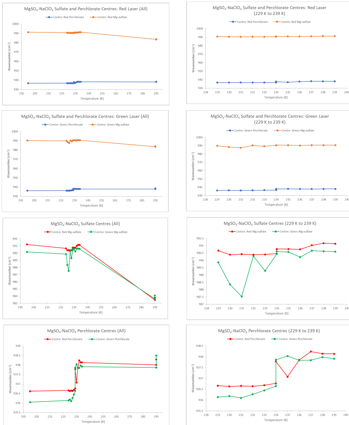
Figure A33: The peak positions of the main sulfate and perchlorate peaks for the MgSO_4-NaClO_4 brine using both the 532 nm and 785 nm lasers.
