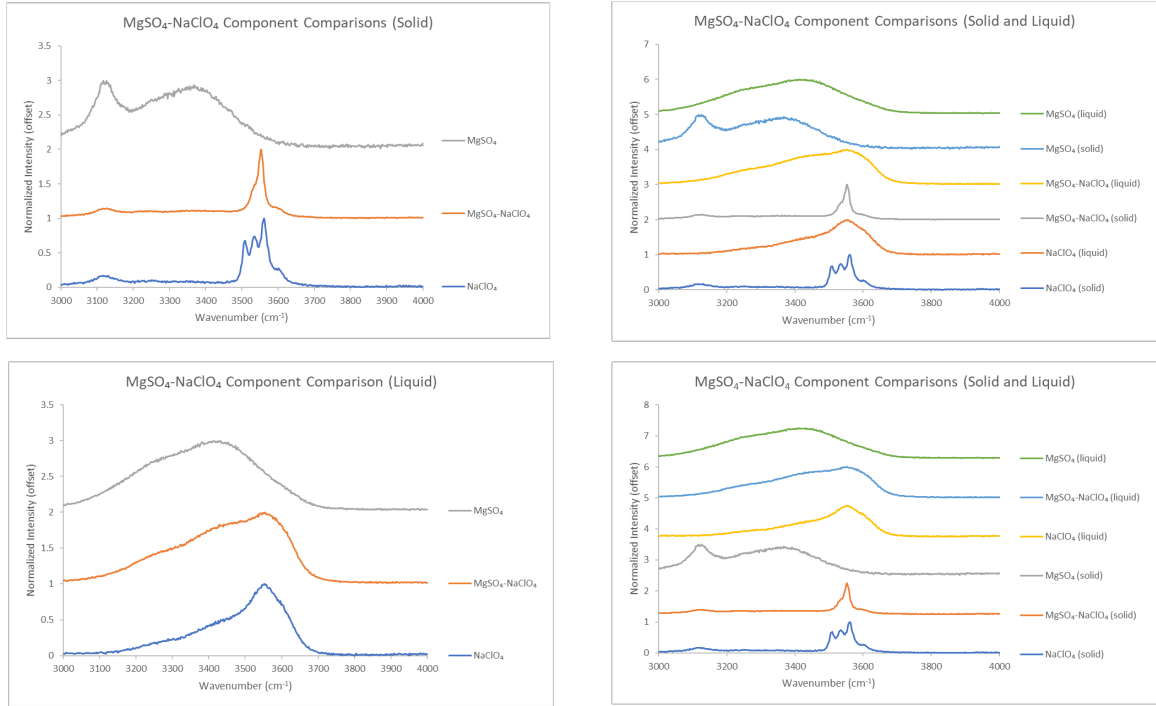
Figure A26: MgSO 4 -NaClO 4 comparison stacked plots between solid (200 K) and liquid (295 K) components of both endmembers and their respective mixed brine using the 532 nm green laser.
