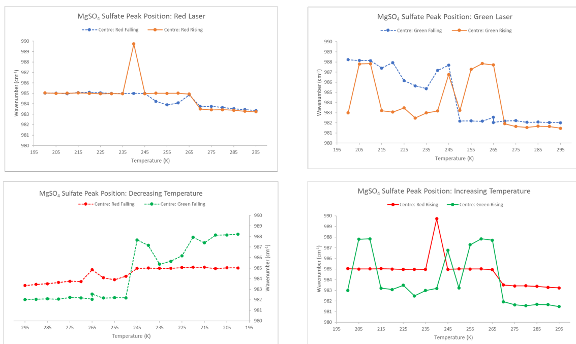
Figure A30: The peak position of the main sulfate peak for magnesium sulfate using both the 532 nm and 785 nm lasers. Note that plots denoting falling temperatures are denoted by dashed lines, while rising temperatures are denoted by solid lines.
