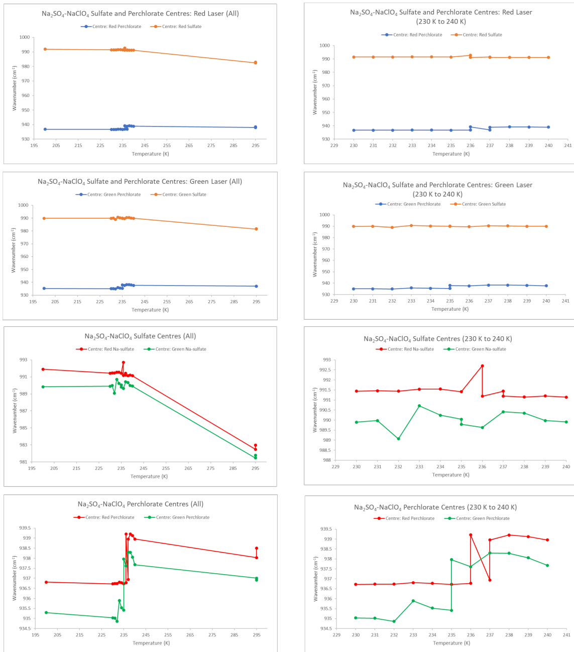
Figure A35: The peak positions of the main sulfate and perchlorate peaks for the Na 2 SO 4 -NaClO 4 brine using both the 532 nm and 785 nm lasers.
