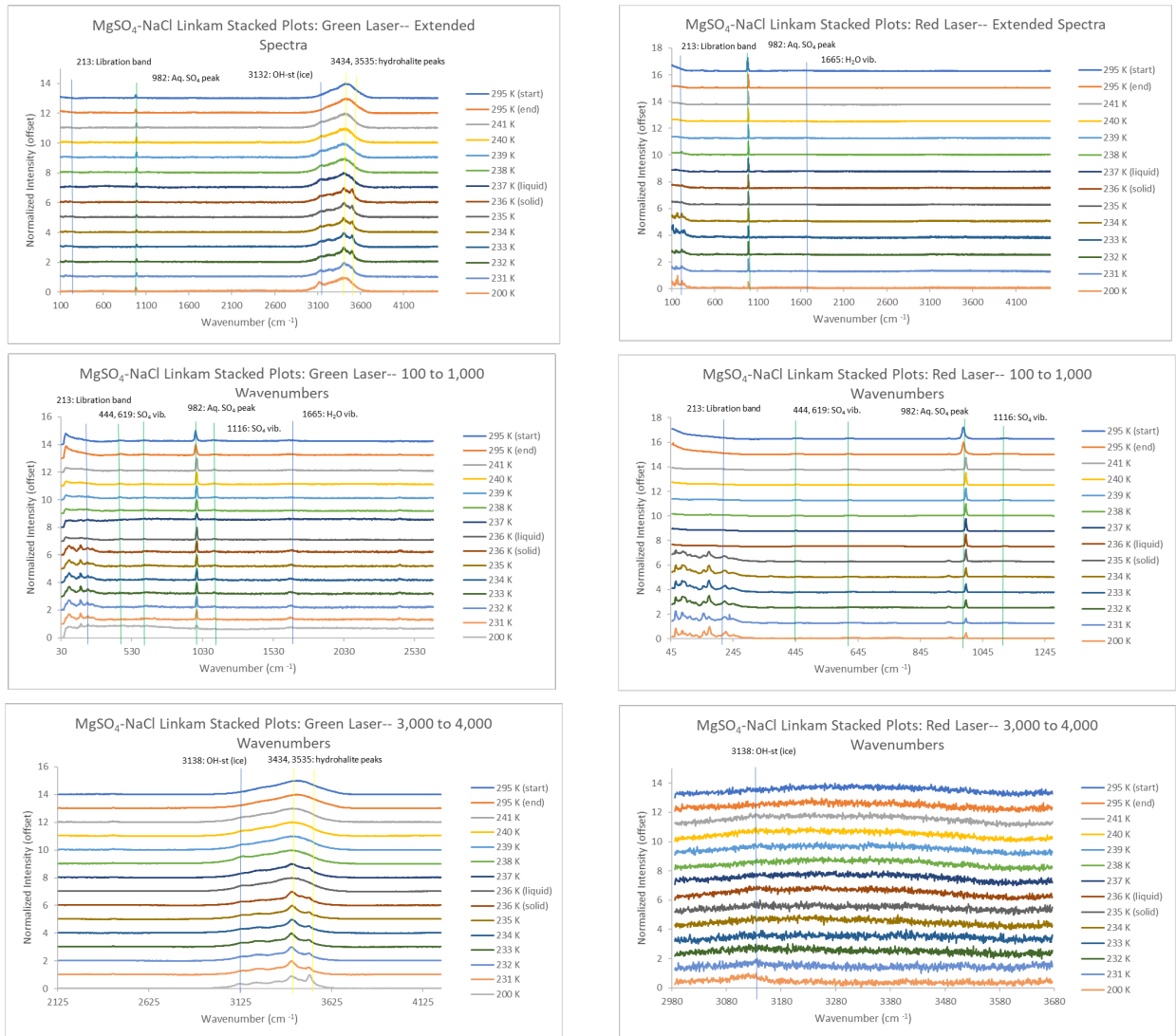
Figure A9: MgSO_4 - NaCl stacked plots (532 nm and 785 nm lasers), lines and labels included to denote important peaks of ultrapure water (light blue), MgSO_4 (dark green), and NaCl (yellow).
