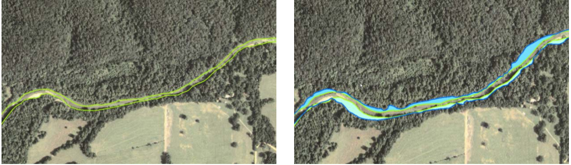
Figure 2.3. Left and right bank (green lines) for Spavinaw Creek on the 2003 NAIP aerial image (left), and creation of polygons (shaded blue area) to determine erosion from 2003-2008 along Spavinaw Creek (right) using ArcGIS.
