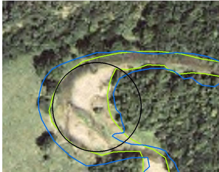
Figure 2.4. Measuring the meander radius of curvature and retreat length using ArcGIS.
