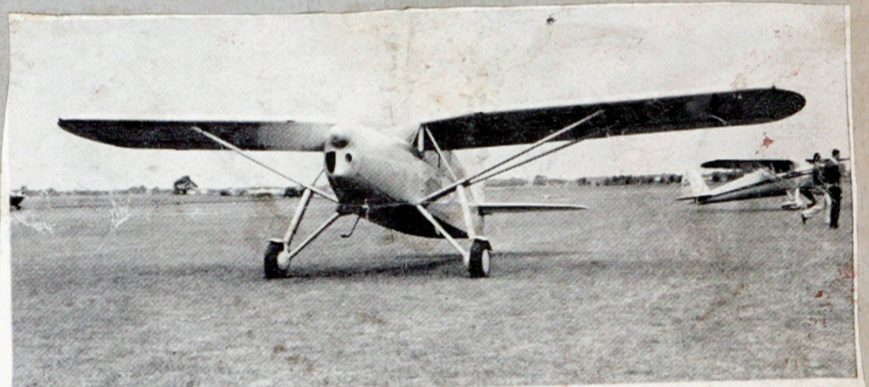
Warner-powered Fairchild "24," with a cruising speed of 122 m.p.h. and a cruising range of 720 costs approximately $6,000. William F. ...
