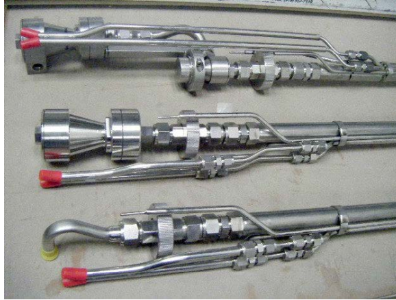
Figure 9. Sampling heads for Method 201A with PM 10 and PM 2.5 sizing cyclones (top), Method 201A with PM 10 sizing cyclone (middle), and Method 17 (bottom) (Buser et al., 2012b).
