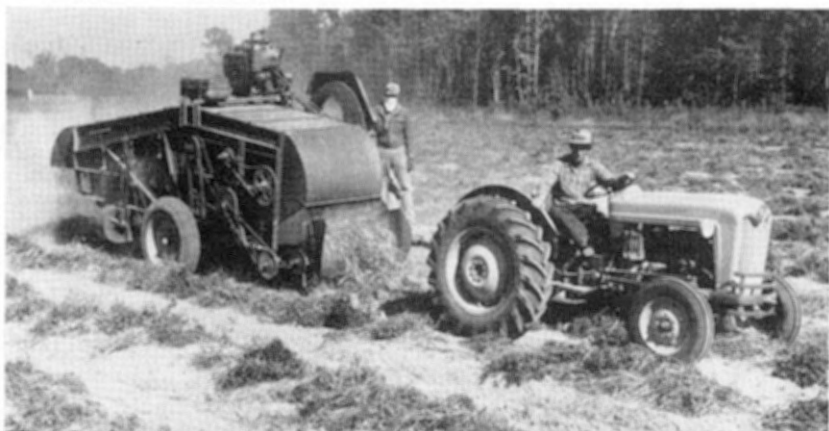
This is another type of combine used for picking peanuts direct from the windrows. Stacking and threshing operations are less efficient than combining.
